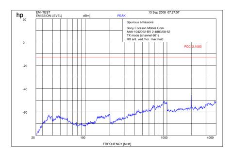
f < 1 GHz : RBW/VBW: 100 kHz Carrier suppressed with a rejection filter  $f \ge 1GHz$  : RBW / VBW 1 MHz
