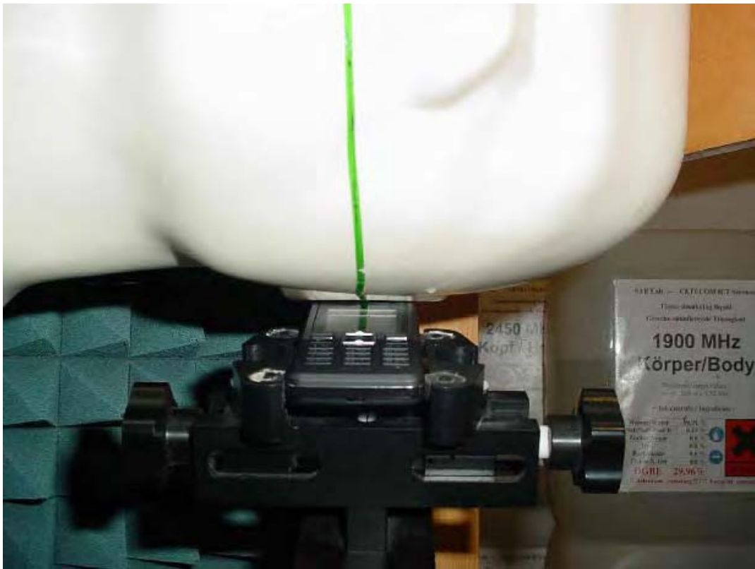
Photo 12: Test position left hand tilted 15°
