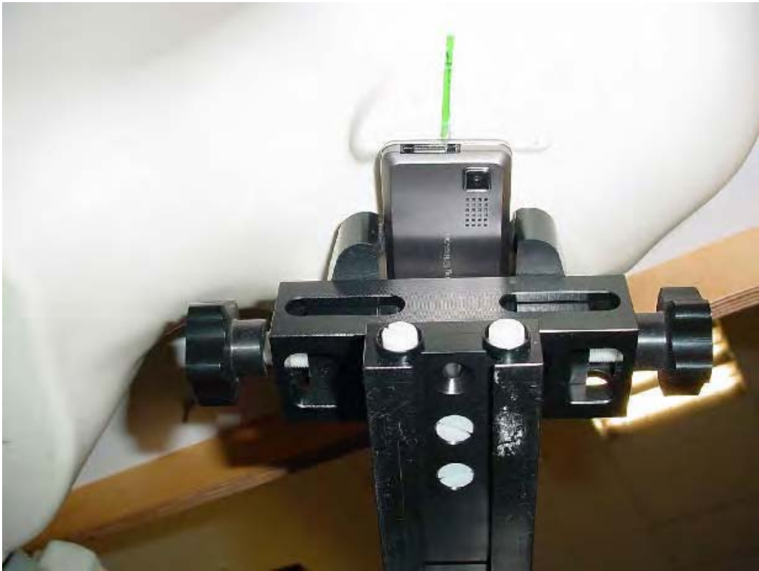
Photo 16: Test position right hand tilted 15°
