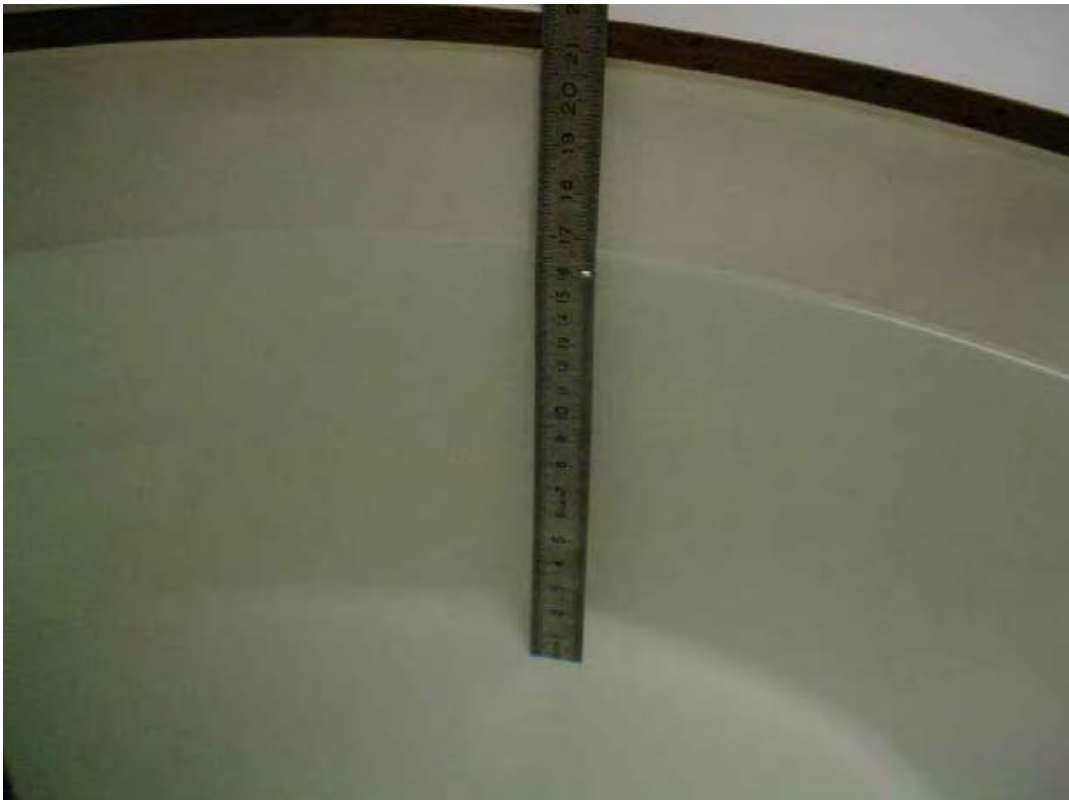
Photo 25: Liquid depth 1900 MHz body simulating liquid
