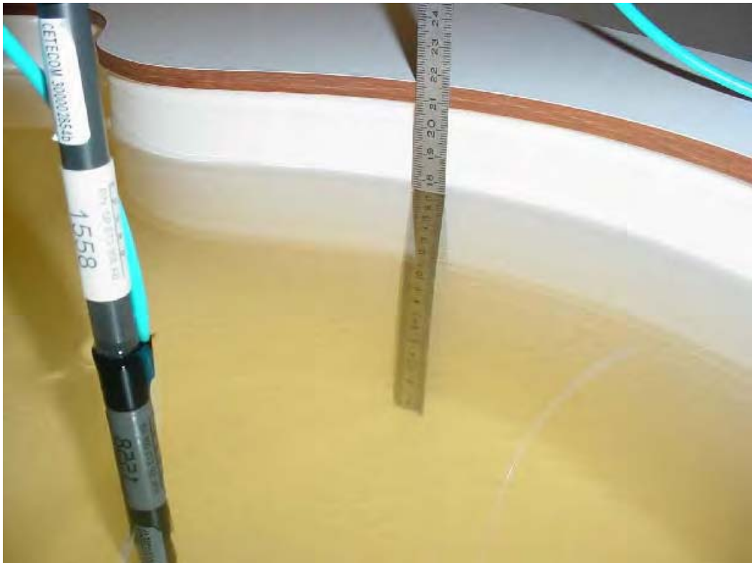
Photo 23: Liquid depth 850 MHz body simulating liquid
