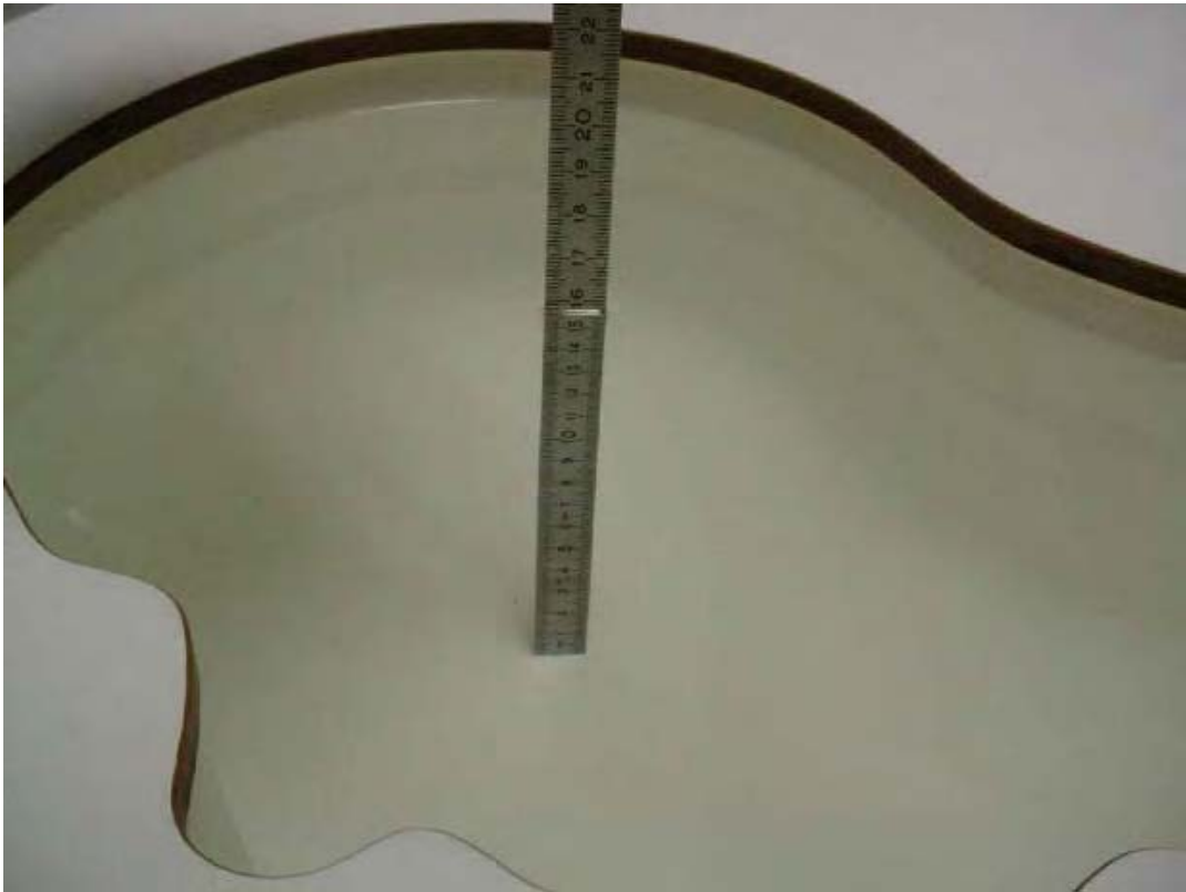
Photo 25: Liquid depth 1900 MHz body simulating liquid
