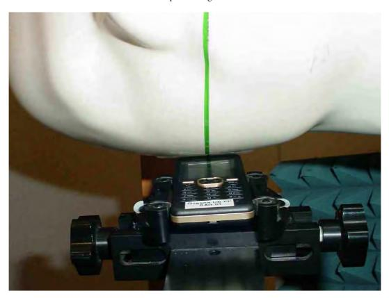
Photo 18: Test position right hand tilted 15°
