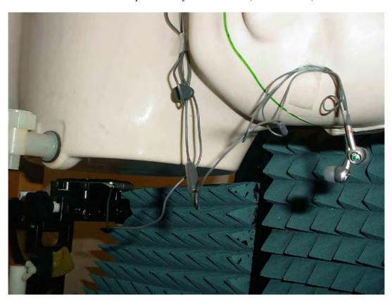
Photo 20: Test position body worn front side (distance 15 mm)
