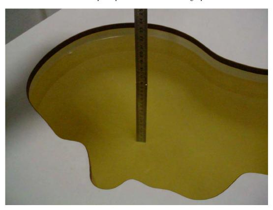
Photo 24: Liquid depth 850 MHz body simulating liquid
