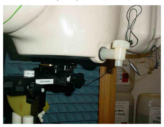
Photo 22: Test position body worn rear side (distance 15 mm)
