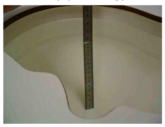
Photo 26: Liquid depth 1900 MHz body simulating liquid
