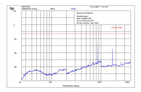
f < 1 GHz : RBW/VBW: 100 kHz Carrier suppressed with a rejection filter
