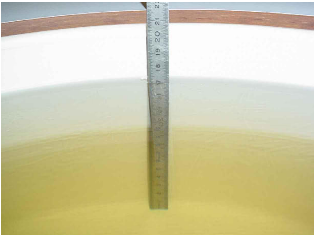
Liquid depth 850 MHz body simulating liquid
