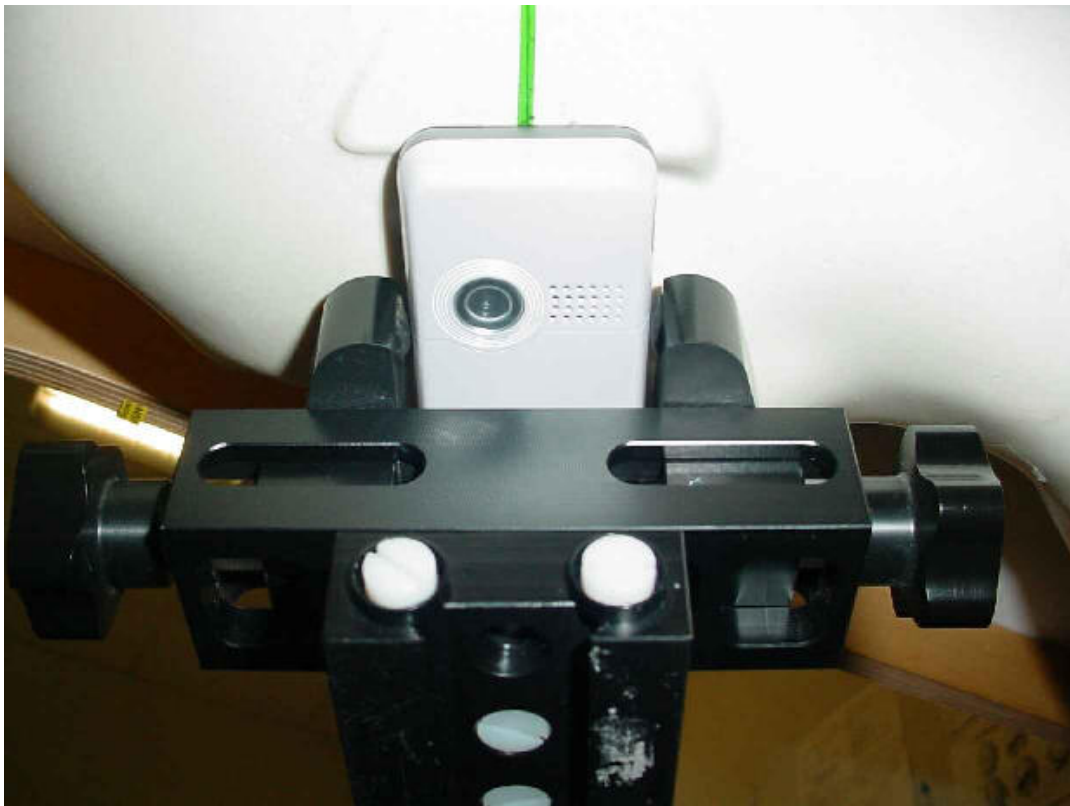
Photo 12: Test position left hand tilted 15°
