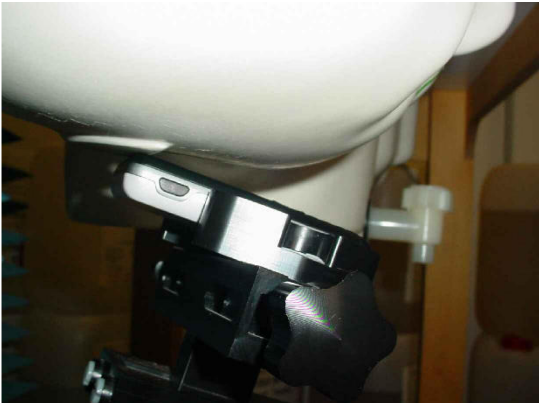
Photo 18: Test position right hand tilted 15°
