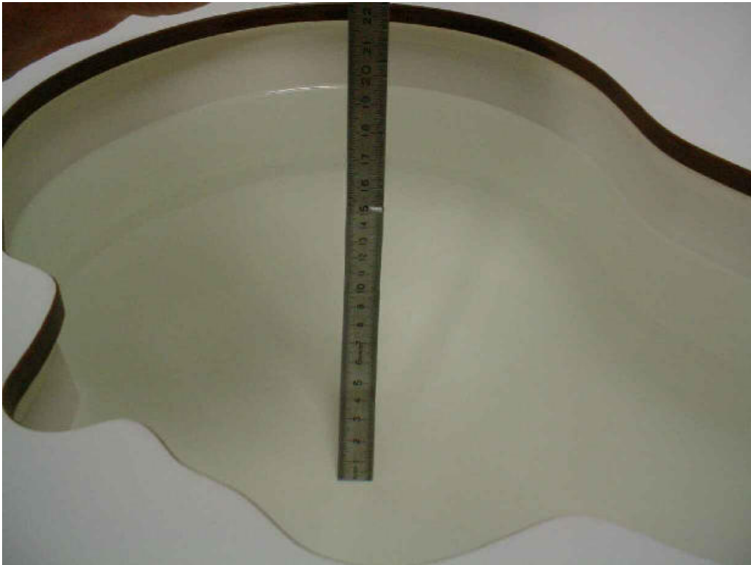
Liquid depth 1900 MHz body simulating liquid
