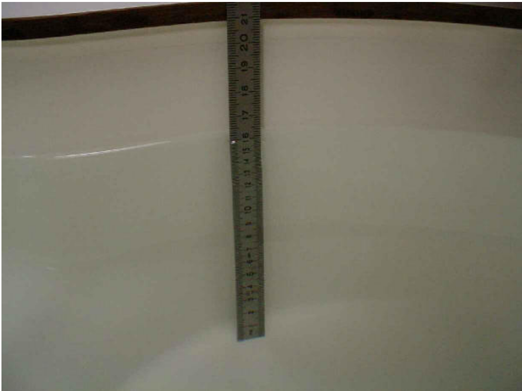
Liquid depth 1900 MHz body simulating liquid
