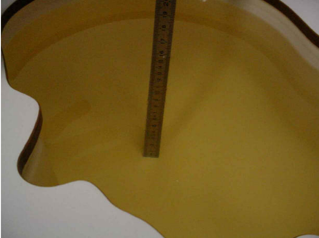
Liquid depth 850 MHz body simulating liquid
