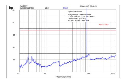
f < 1 GHz: RBW/VBW: 100 kHz  $f \ge 1 \text{GHz}: RBW / VBW 1 \text{ MHz}$  Carrier suppressed with a rejection filter
