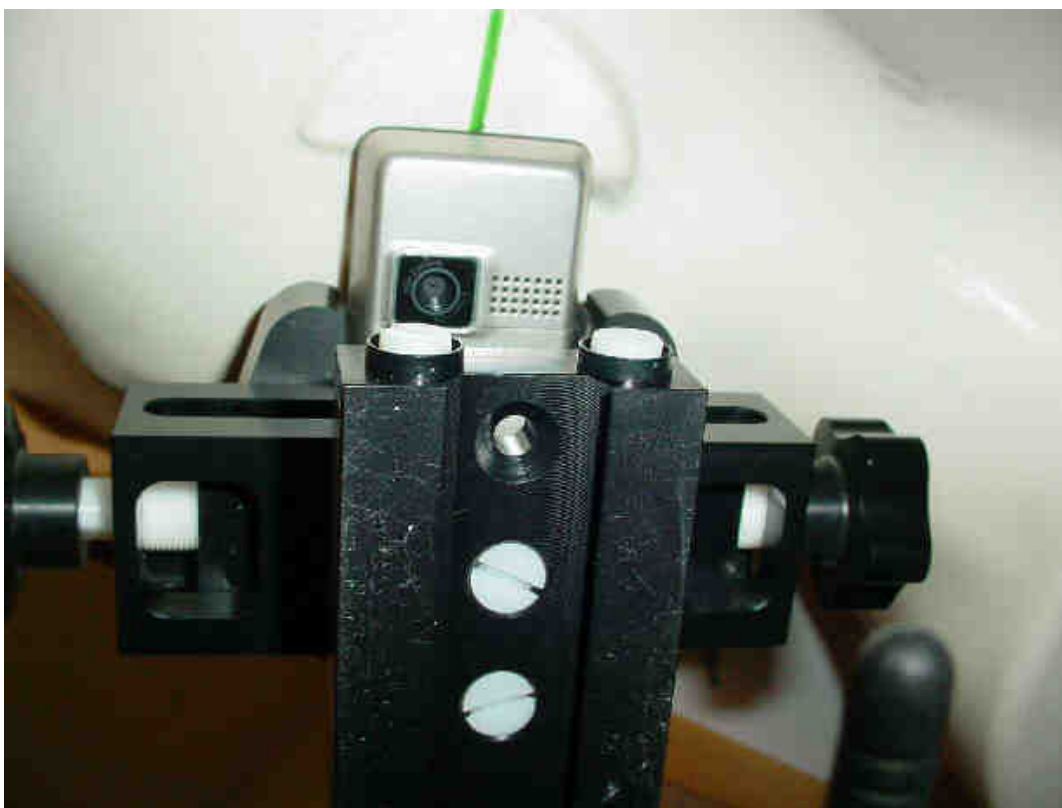
Photo 15: Test position right hand touched
