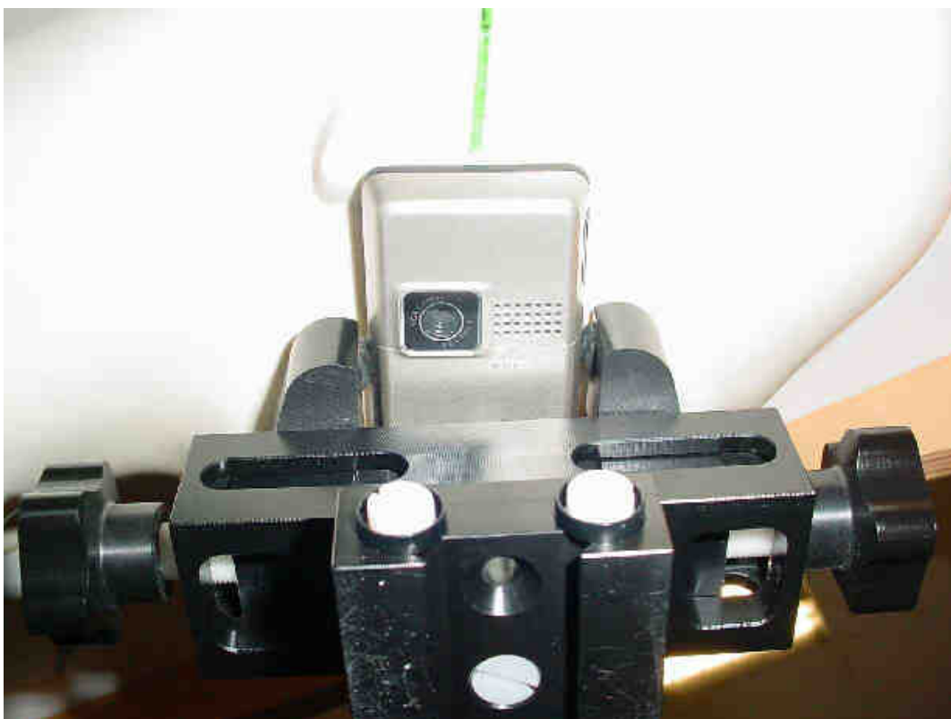
Photo 17: Test position right hand touched
