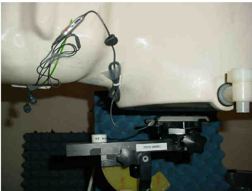
Photo 23: Test position body worn rear side (distance 15 mm)
