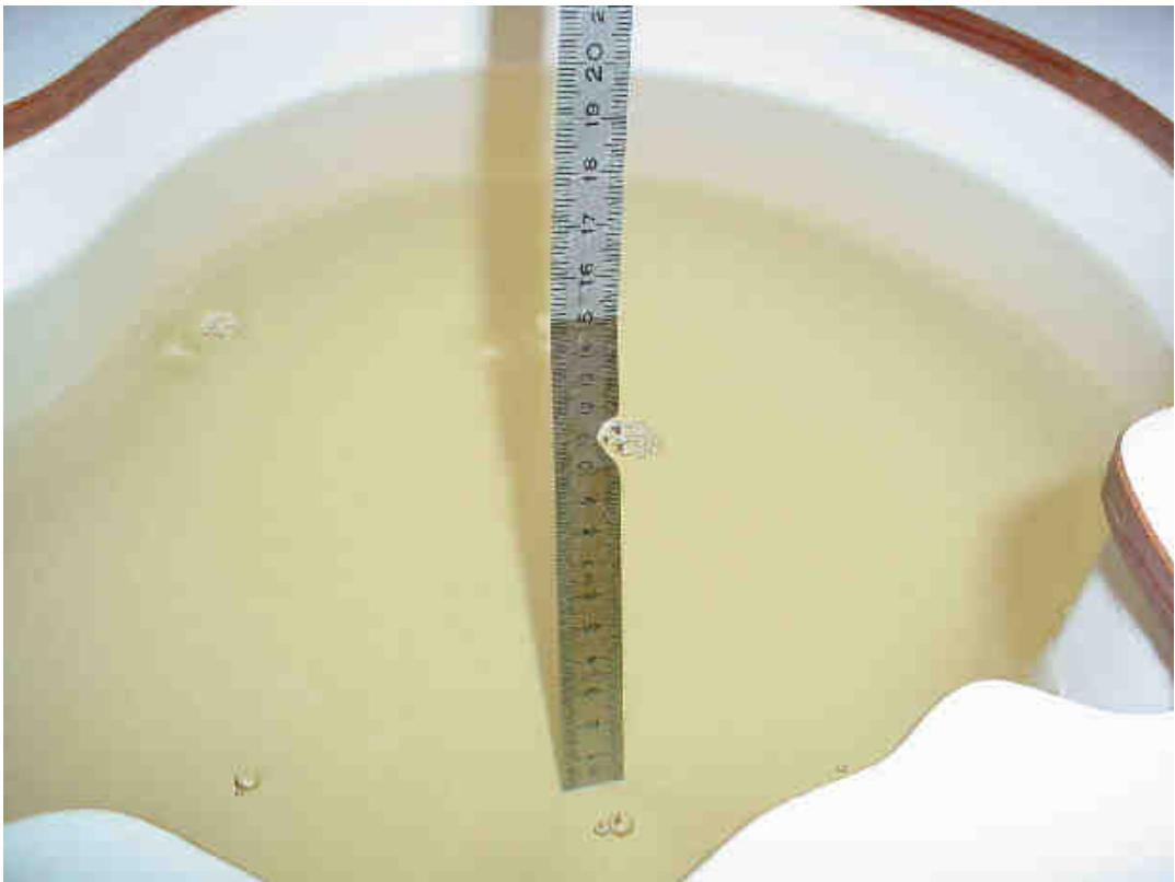
Photo 25: Liquid depth 850 MHz body simulating liquid
