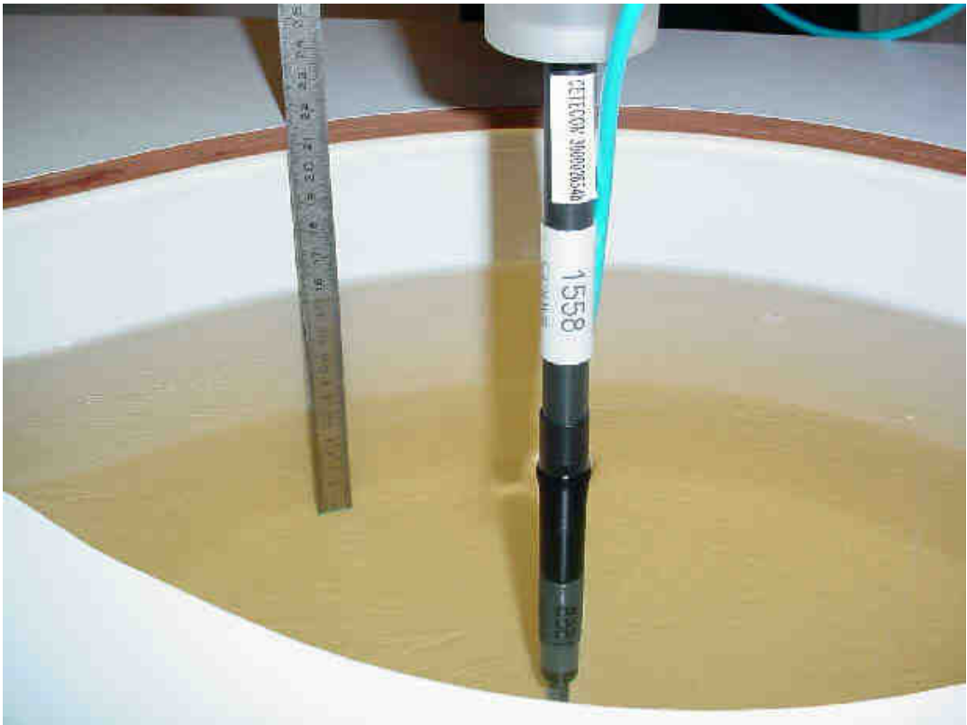
Photo 25: Liquid depth 850 MHz body simulating liquid
