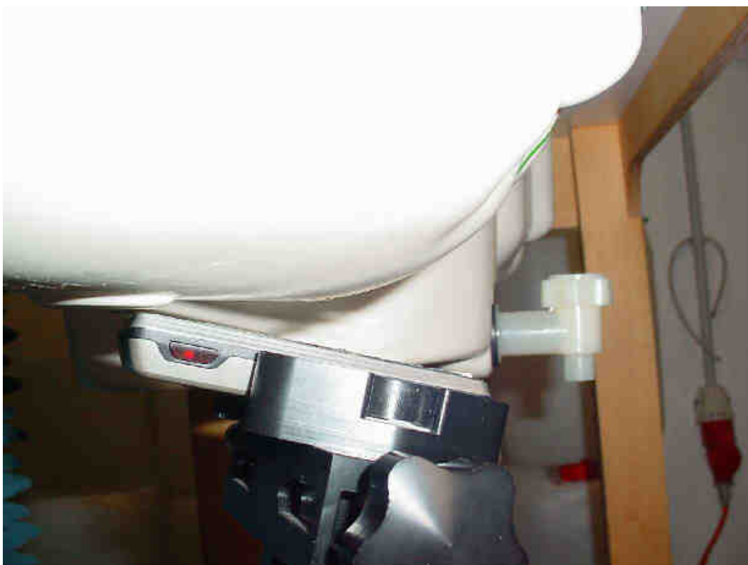
Photo 19: Test position right hand tilted 15°
