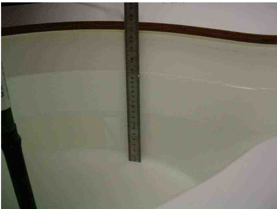
Photo 27: Liquid depth 1900 MHz body simulating liquid
