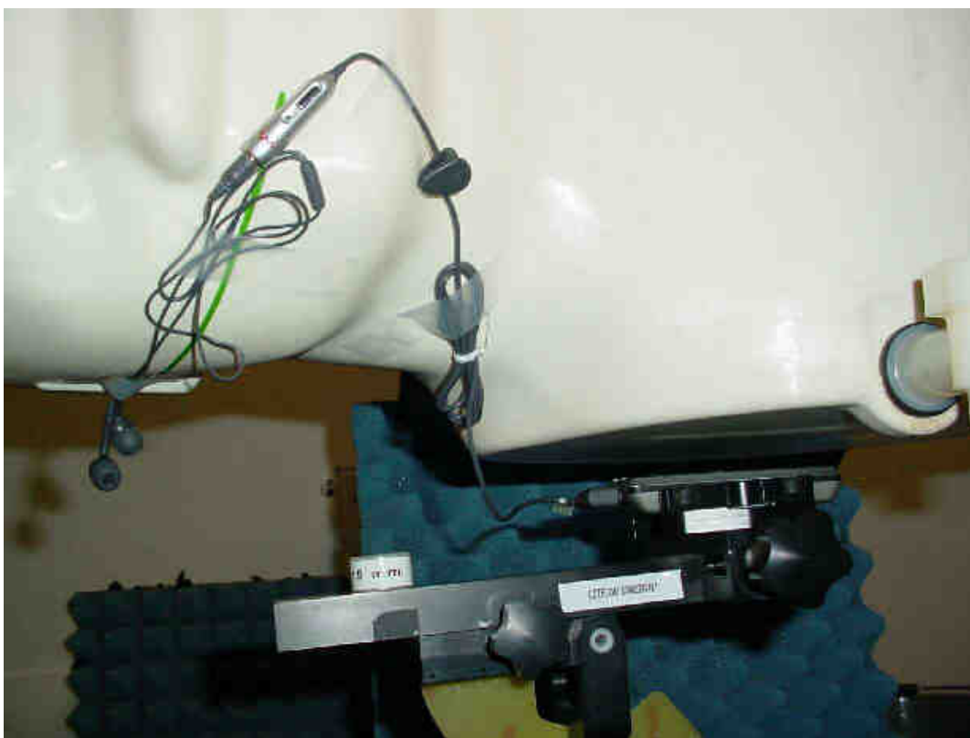
Photo 21: Test position body worn front side (distance 15 mm)
