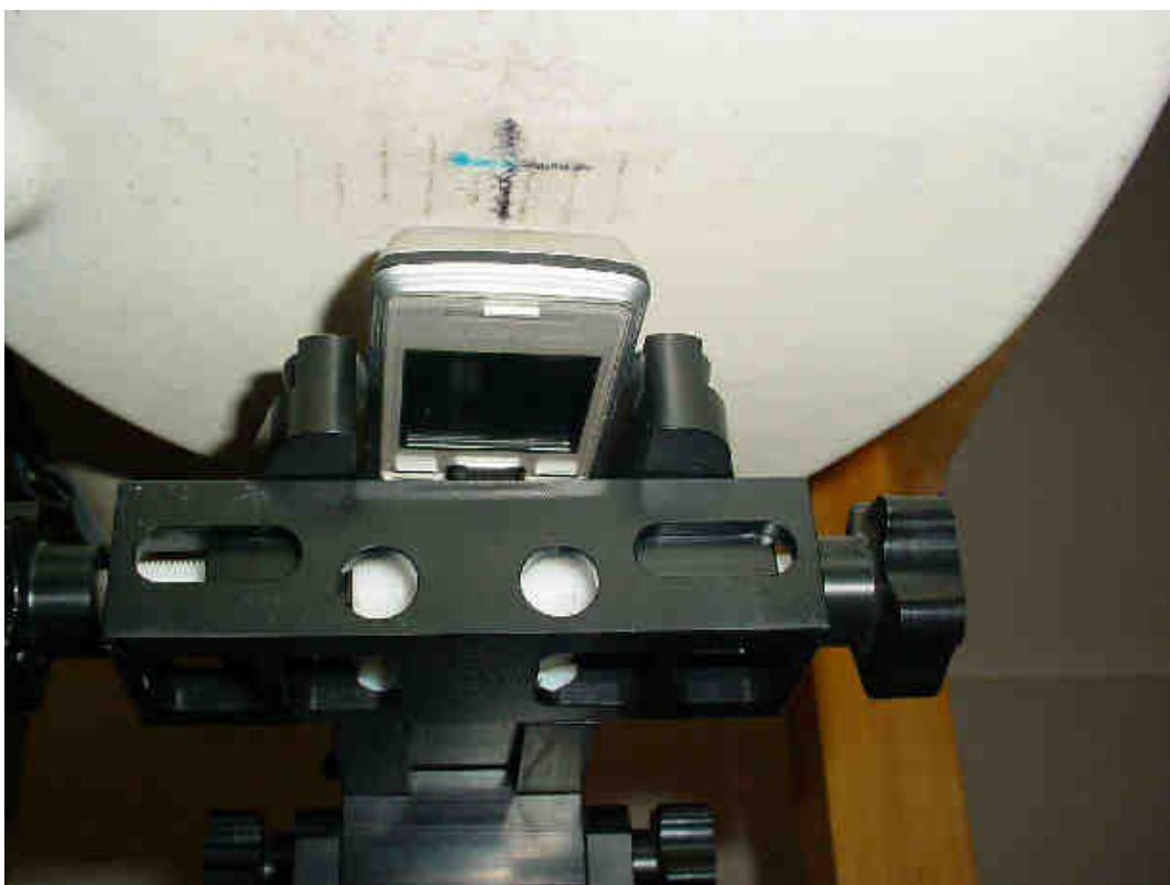
Photo 23: Test position body worn rear side (distance 15 mm)
