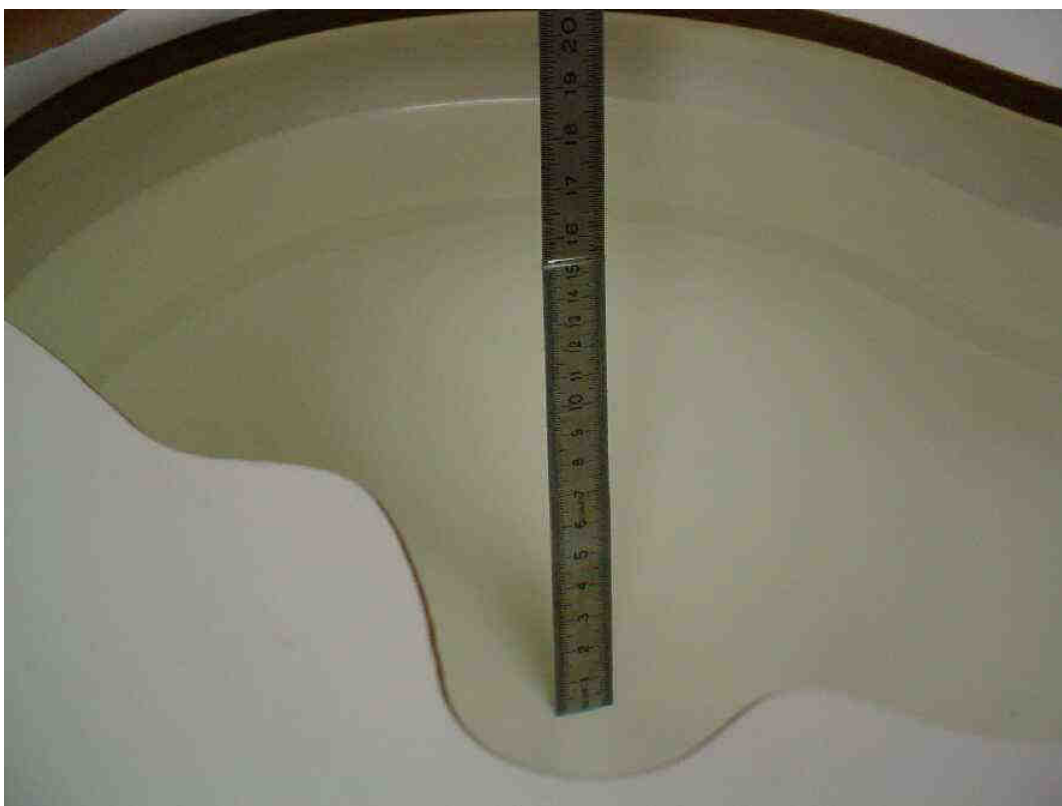
Photo 27: Liquid depth 1900 MHz body simulating liquid
