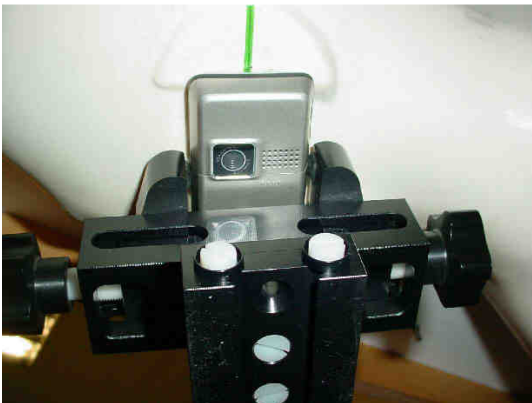
Photo 11: Test position left hand touched
