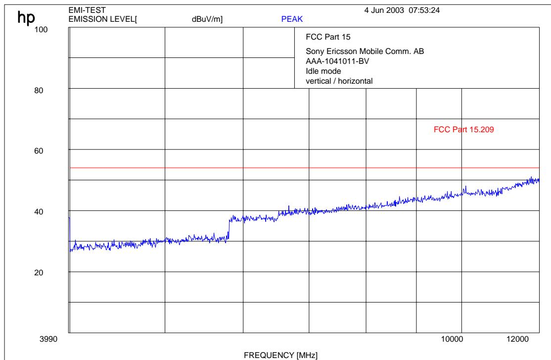
**f < 1 GHz : RBW/VBW: 100 kHz****f ≥ 1GHz : RBW/VBW 1 MHz****REFERENCE NUMBER(S) OF TEST EQUIPMENT USED****(for reference numbers see test equipment listing)****17 – 24, 64; 52-63**
