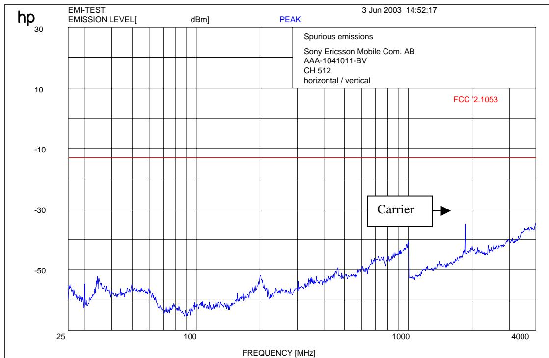
**$f < 1 \text{ GHz}$  : RBW/VBW: 100 kHz** **$f \geq 1 \text{ GHz}$  : RBW / VBW 1 MHz****Carrier suppressed with a rejection filter****REFERENCE NUMBER(S) OF TEST EQUIPMENT USED****(for reference numbers see test equipment listing)****17 – 24; 64**
