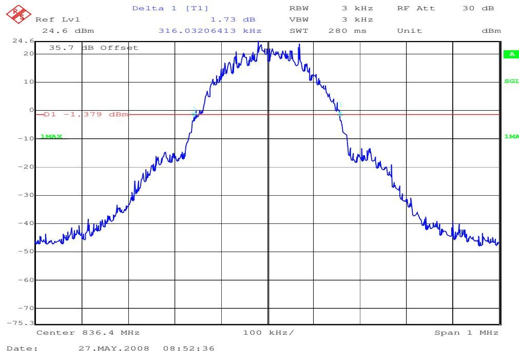
**Channel 251****99% (-20 dB) Occupied Bandwidth**
