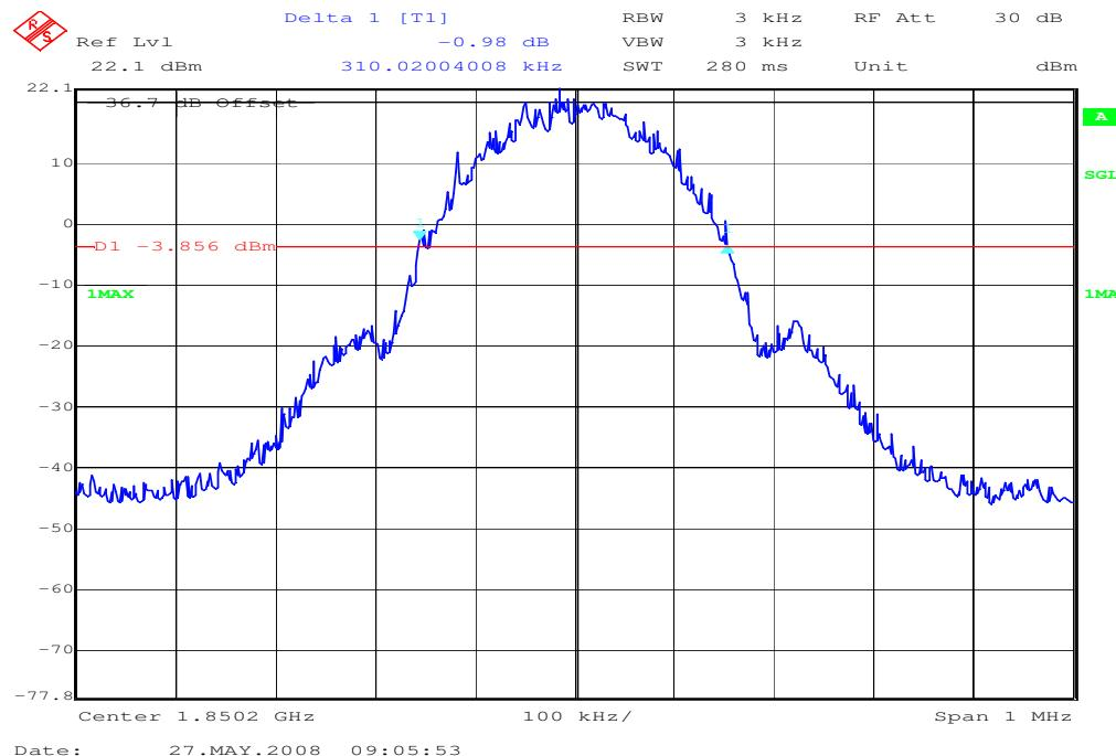
**Channel 661****99% (-20 dB) Occupied Bandwidth**
