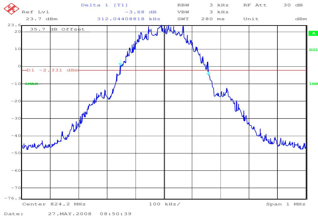
**Channel 189****99% (-20 dB) Occupied Bandwidth**
