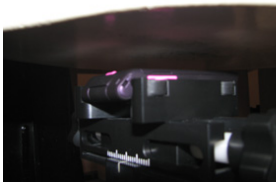
Device position against the body: Phone on 15mm distance against Phantom
