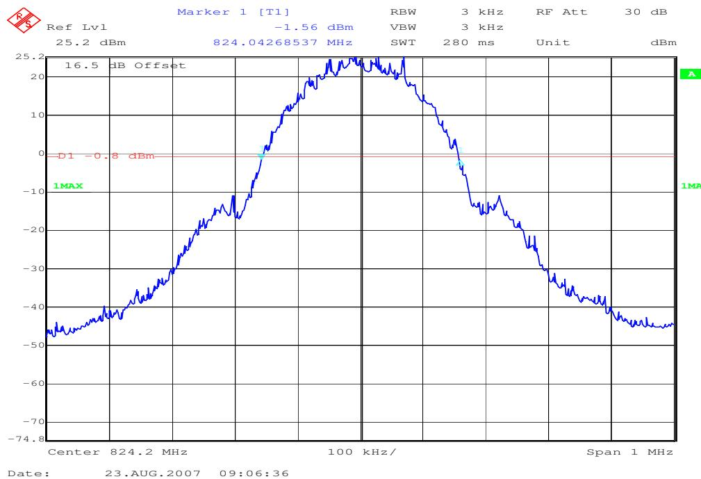
**Channel 189****99% (-20 dB) Occupied Bandwidth**
