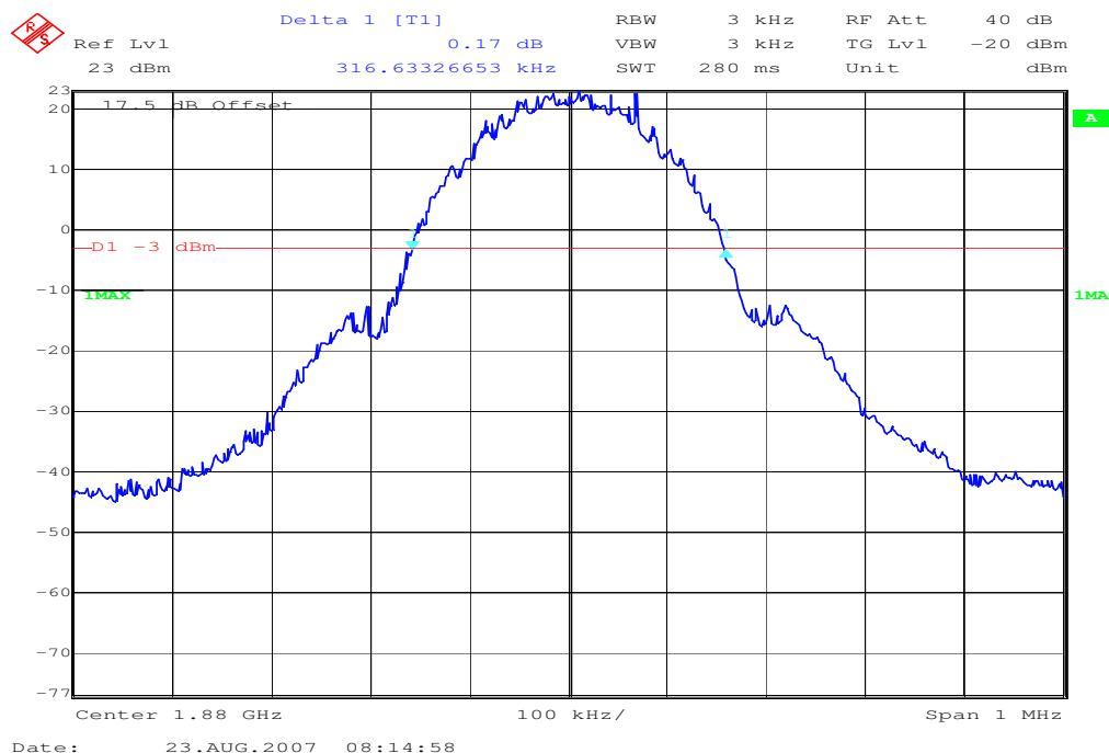
**Channel 810****99% (-20 dB) Occupied Bandwidth**
