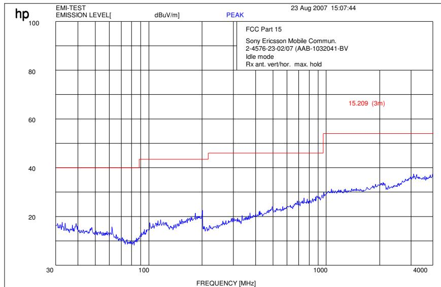
$f < 1 \text{ GHz}$  : RBW/VBW: 100 kHz $f \geq 1 \text{ GHz}$  : RBW / VBW 1 MHz**IDLE-MODE (4 GHz – 12.0 GHz)**
