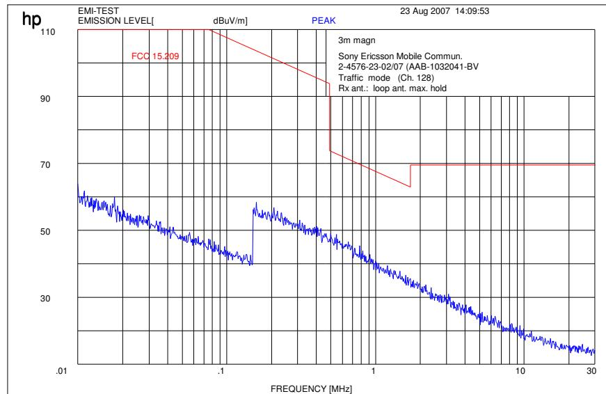
**Channel 128 (30 MHz - 4 GHz)**
