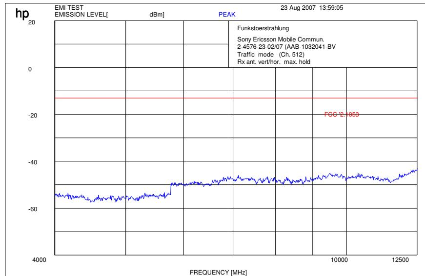
$f < 1 \text{ GHz}$  : RBW/VBW: 100 kHz $f \geq 1 \text{ GHz}$  : RBW / VBW 1 MHz**Channel 512 (12 GHz - 25 GHz) valid for all 3 channels**
