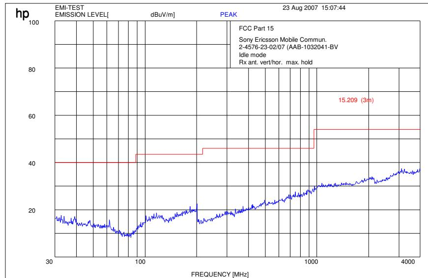
$f < 1 \text{ GHz}$  : RBW/VBW: 100 kHz $f \geq 1 \text{ GHz}$  : RBW / VBW 1 MHz**Idle Mode (4 GHz – 12.0 GHz)**
