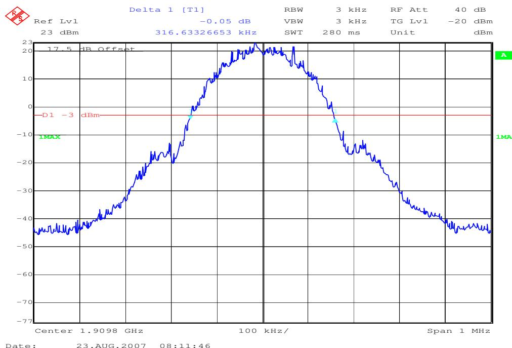
**Channel 661****99% (-20 dB) Occupied Bandwidth**
