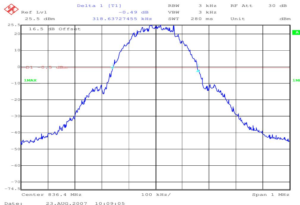
**Channel 251****99% (-20 dB) Occupied Bandwidth**
