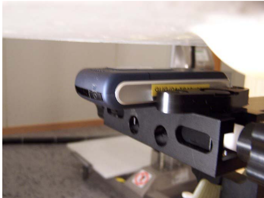
Device position against the body: Phone's back to the phantom without HF
