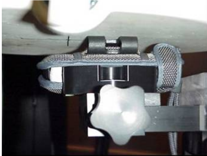
Position of device against flat phantom using carry accessory ICT-14 with hands free accessory RLF 501 25/04 (HPE-14).
