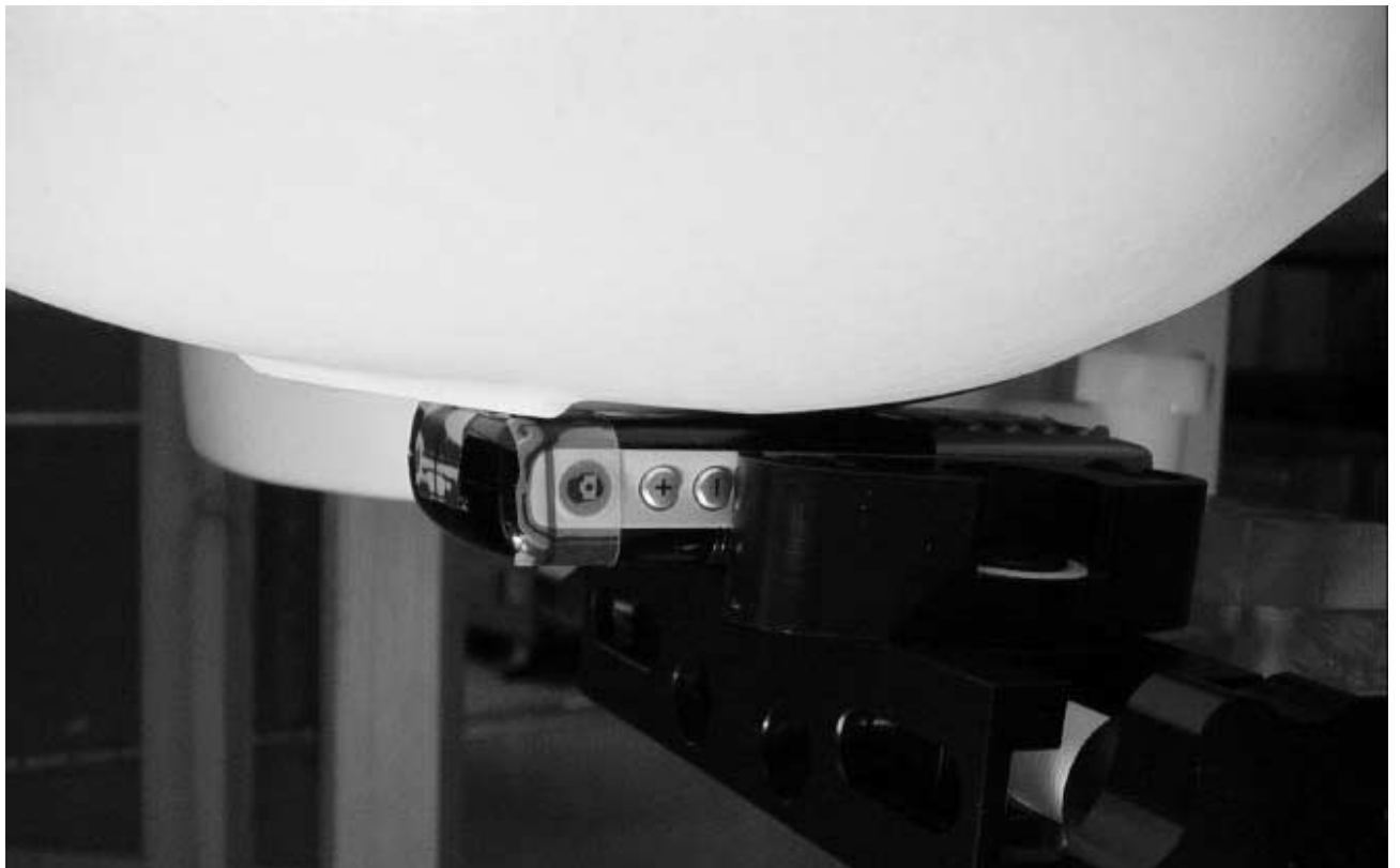
Position of device against head phantom using the “cheek” position
