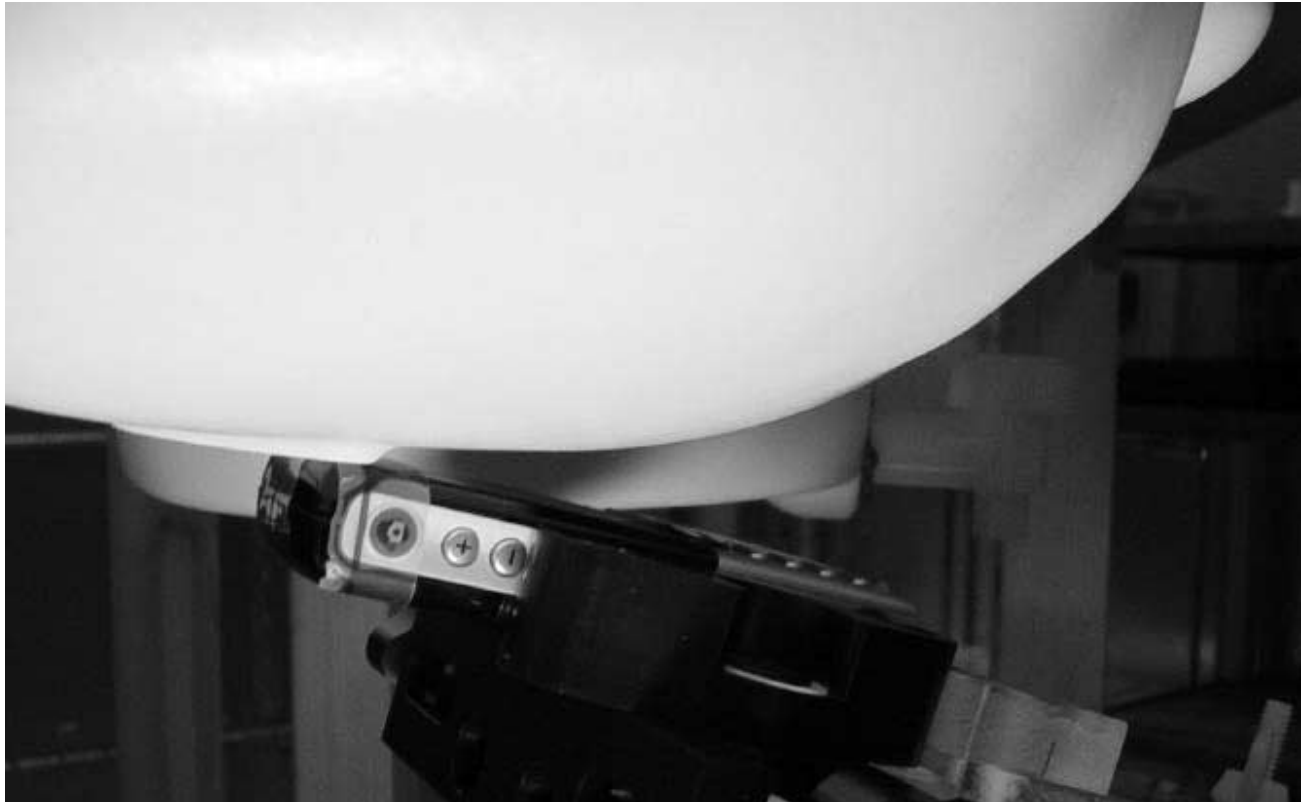
Position of device against head phantom using the “tilt” position
