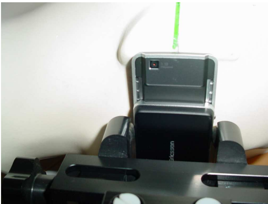
Photo 30: Test position right hand tilted 15° slide opened
