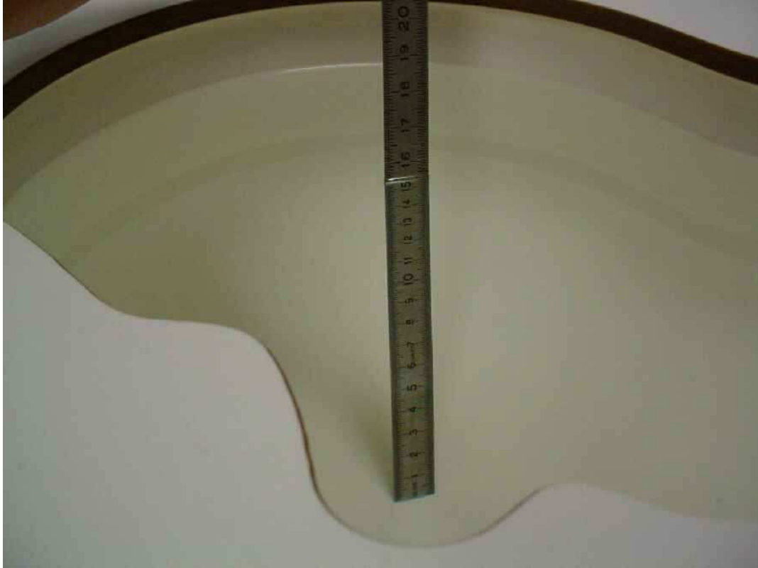
Photo 36: Liquid depth 1900 MHz body simulating liquid
