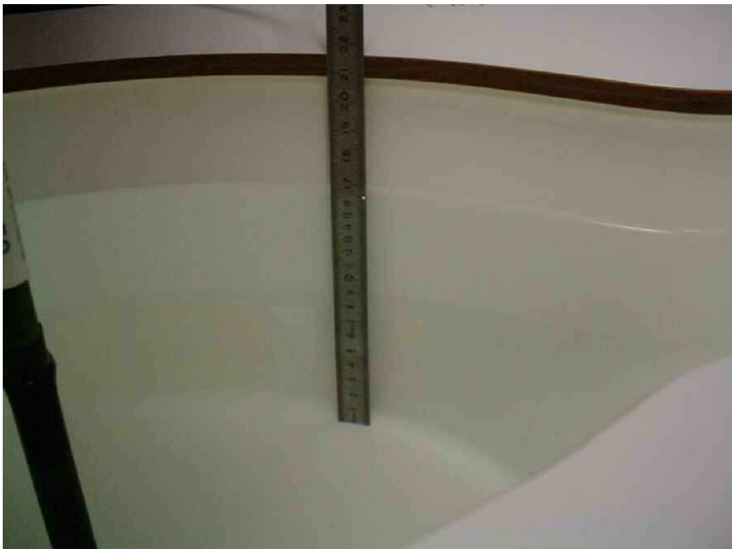
Photo 36: Liquid depth 1900 MHz body simulating liquid
