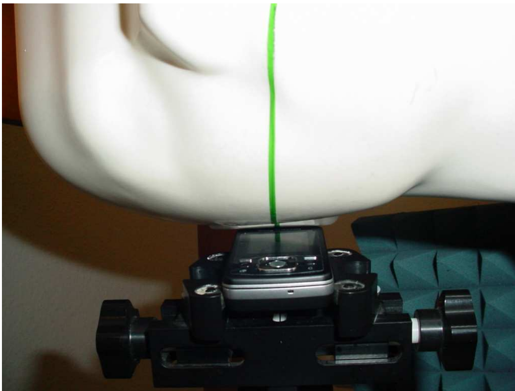
Photo 26: Test position right hand tilted 15°
