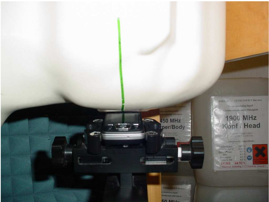
Photo 16: Test position left hand tilted 15°
