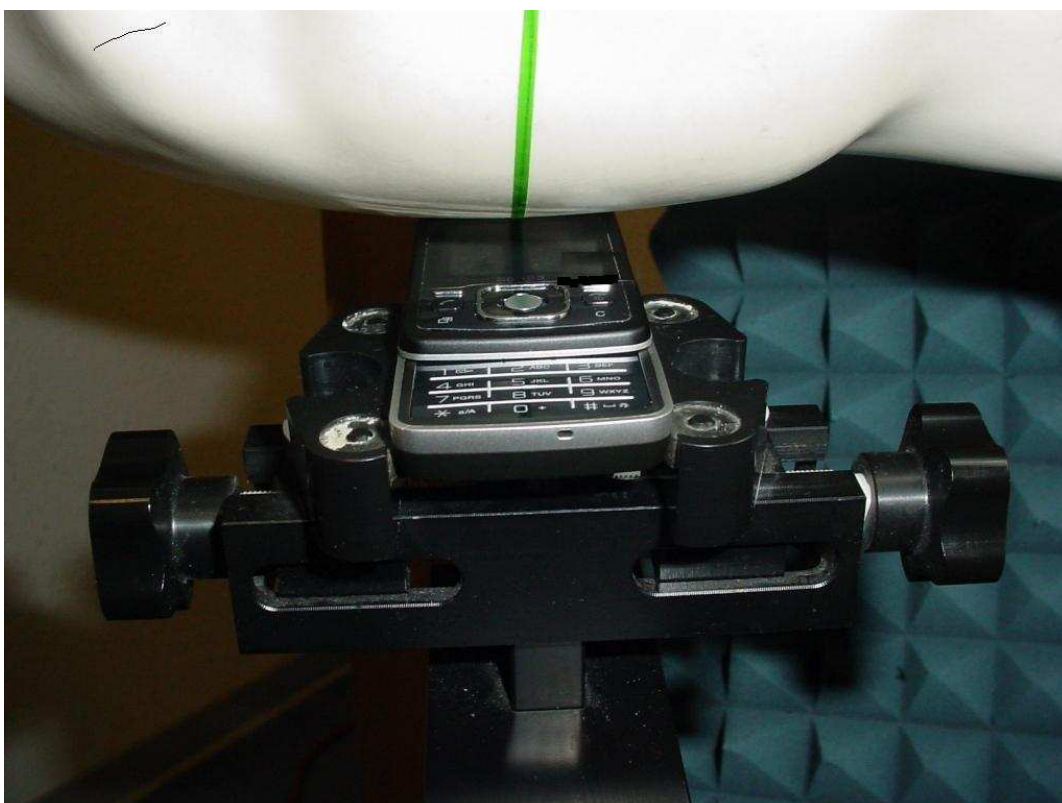
Photo 30: Test position right hand tilted 15° slide opened
