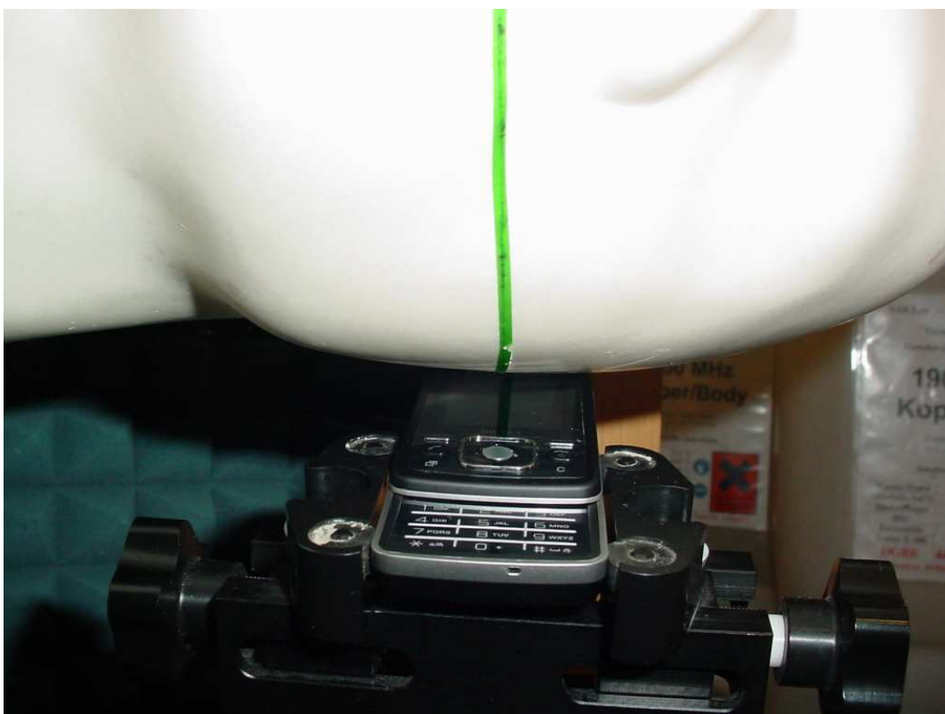
Photo 20: Test position left hand tilted 15° slide opened
