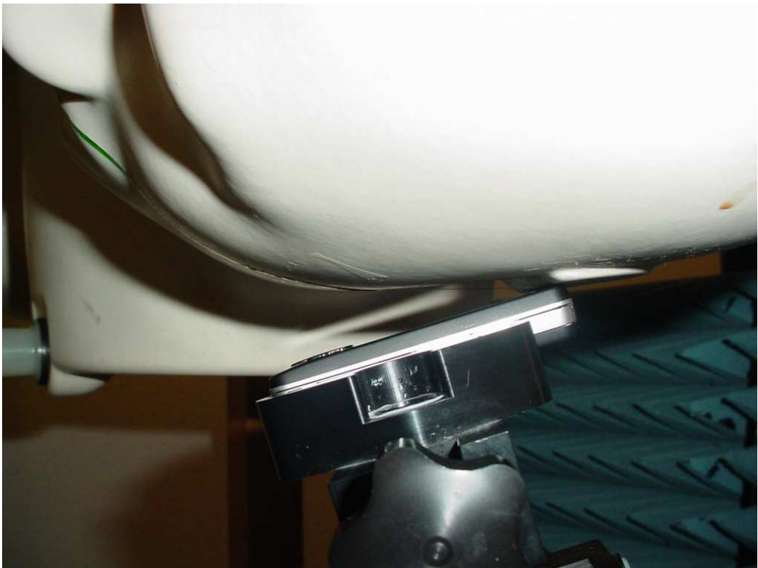
Photo 16: Test position left hand tilted 15°
