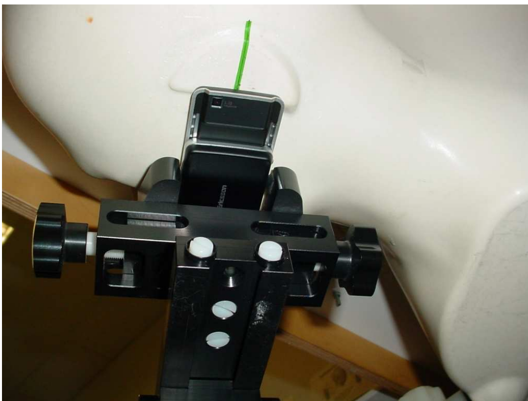
Photo 20: Test position left hand tilted 15° slide opened
