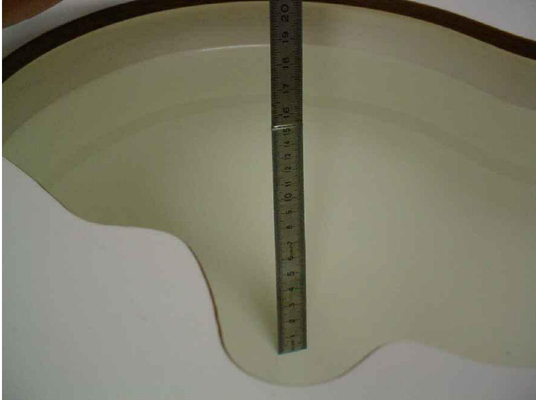
Photo 24: Liquid depth 1900 MHz body simulating liquid
