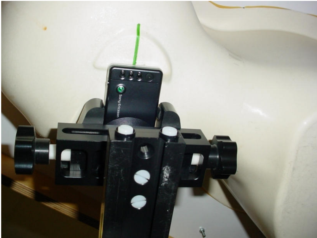
Photo 12: Test position left hand tilted 15°
