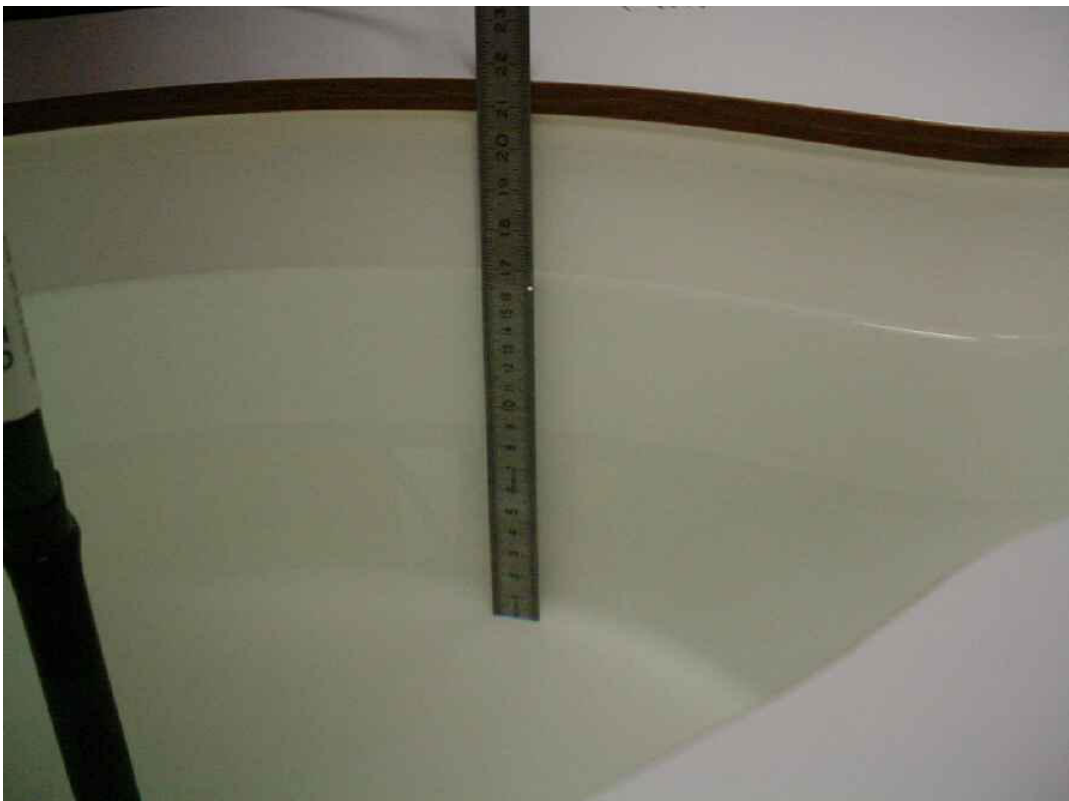
Photo 24: Liquid depth 1900 MHz body simulating liquid
