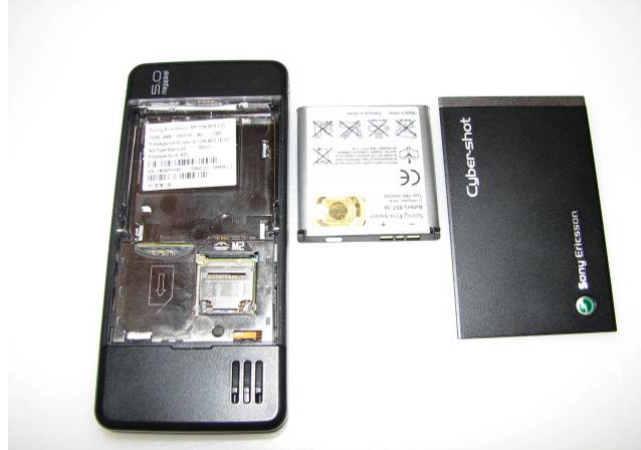
Battery and cover removed
