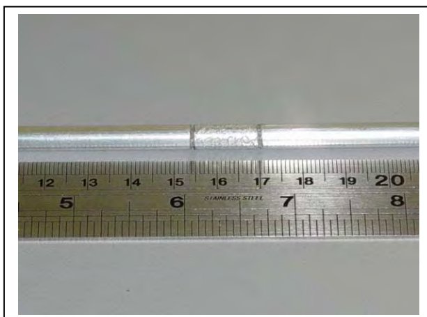
Pictures to show depth gauge used for measuring TSL depth. Note: The low end of the scale is a depth of 15.5 cm.
