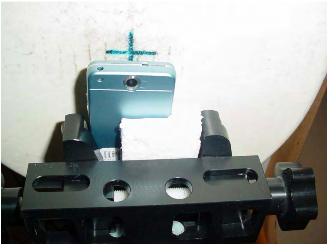
Photo 26: Test position body worn front side (15 mm distance)
