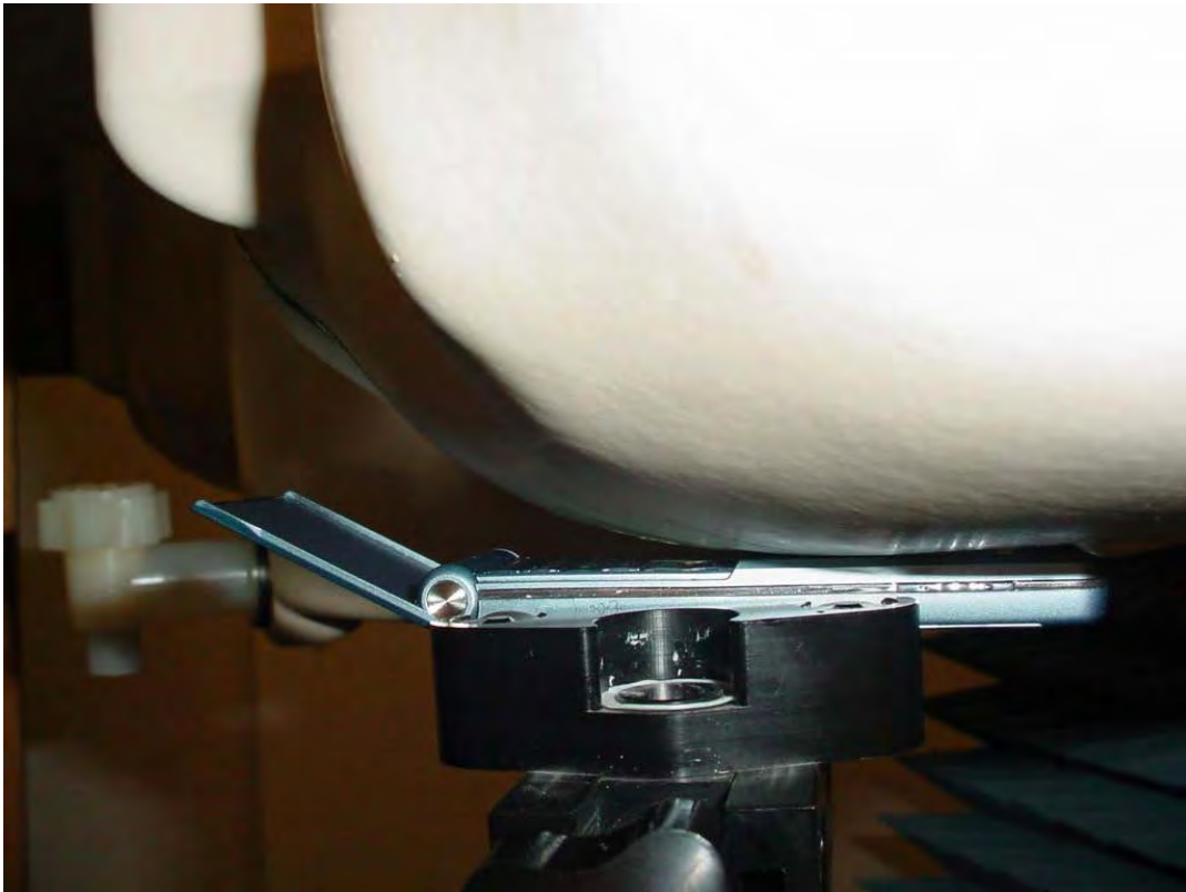
Photo 16: Test position left hand tilted 15°
