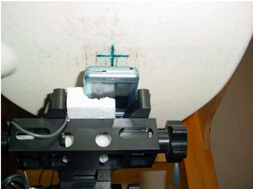
Photo 28: Test position body worn rear side (15 mm distance)
