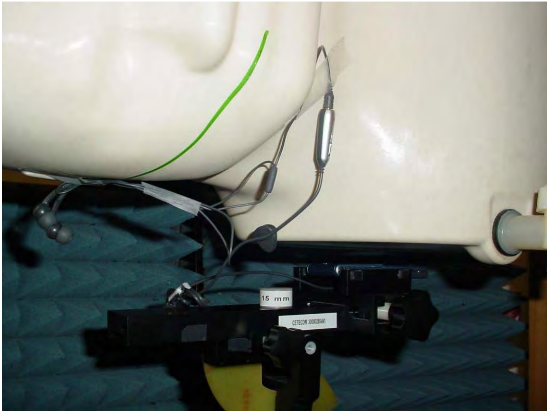
Photo 26: Test position body worn front side (15 mm distance)
