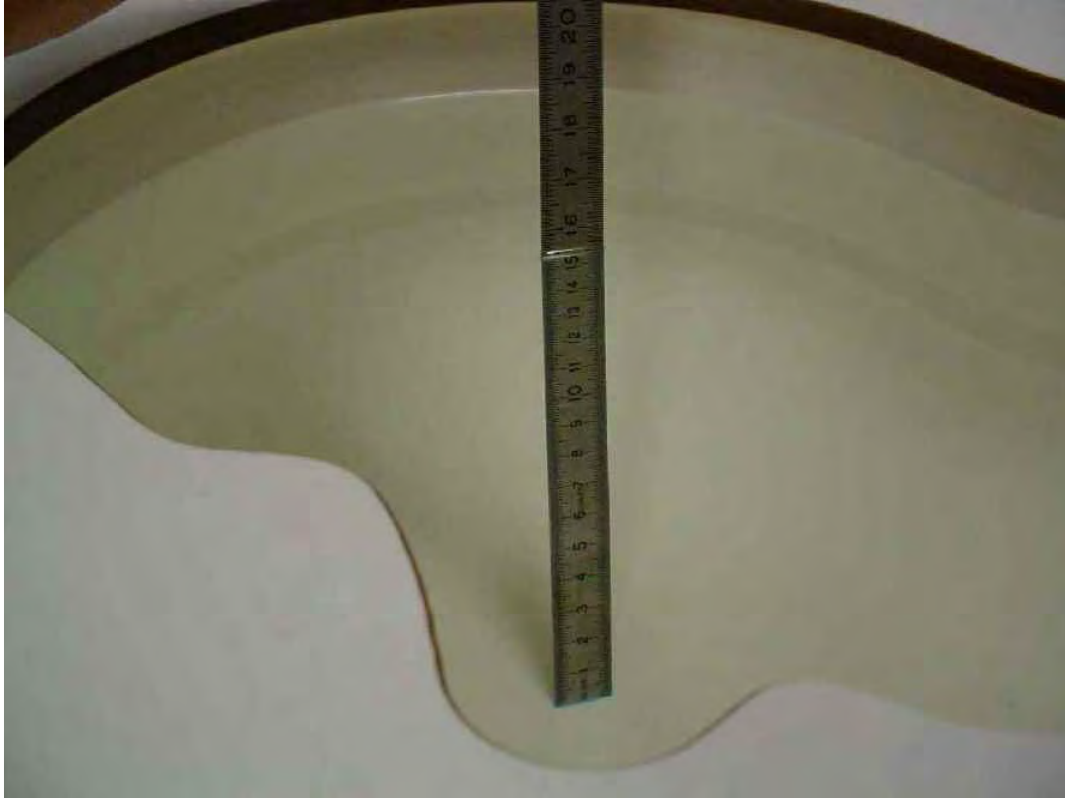
Photo 30: Liquid depth 1900 MHz body simulating liquid
