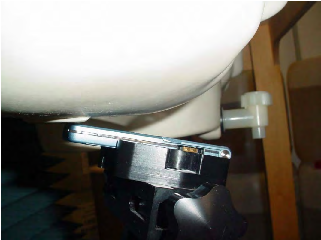
Photo 24: Test position right hand tilted 15°
