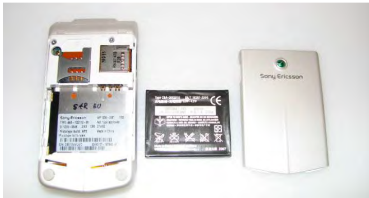
Battery and cover removed
