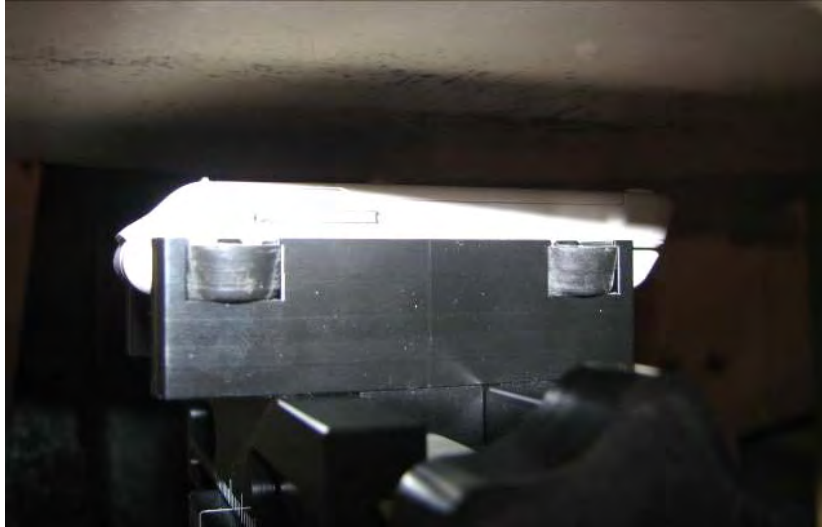
DUT in body position with 15 mm distance
