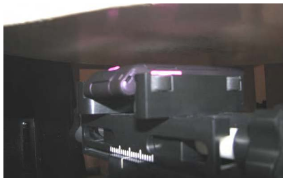
DUT in body position with 15 mm distance
