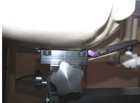
DUT position towards the head: Cheek (touch) position
