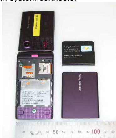
Battery and cover removed
