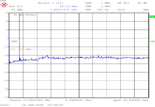
The peak at the left site of the plot is the local oscillator from the spectrum analyzer. No spurious emissions were found.
