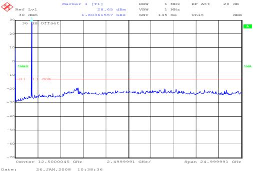
The peak at the left site of the plot is the local oscillator from the spectrum analyzer. No spurious emissions were found.
