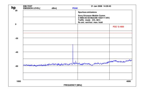
$f \ge 1 GHz : RBW / VBW 1 MHz$ Carrier suppressed with a rejection filter
