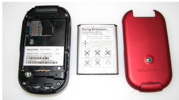
Battery and cover removed
