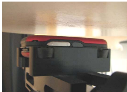
DUT in body position with 15 mm distance
