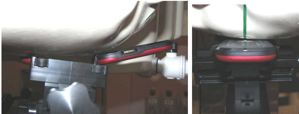
DUT position towards the head: Cheek (touch) position
