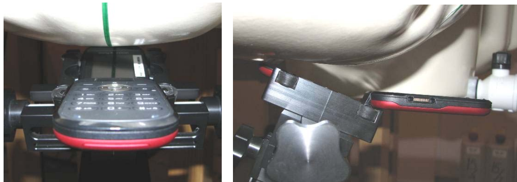
DUT position towards the head: Tilt (touch + 15°) position
