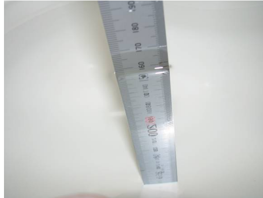
Head liquid depth 168 mm
