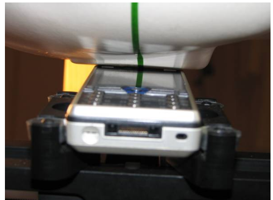
DUT position towards the head: Tilt (touch + 15°) phone position
