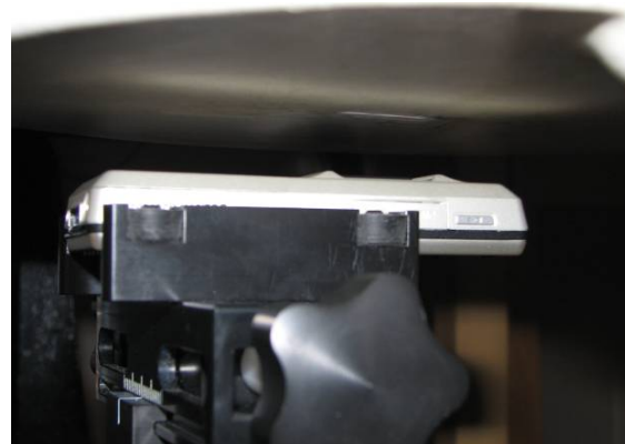
DUT position towards the body: 15 mm distance between SAM and DUT
