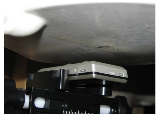
DUT position towards the body: 15 mm distance between SAM and DUT
