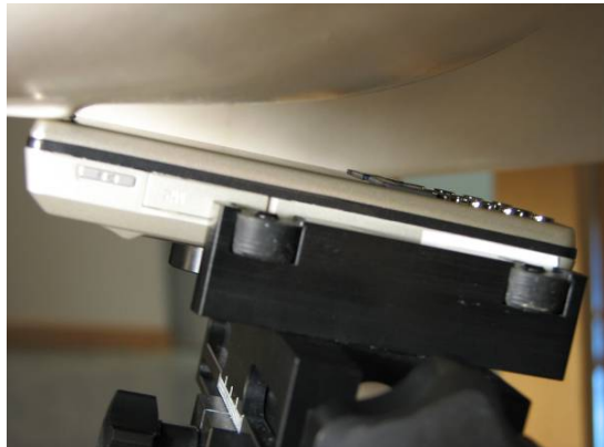
DUT position towards the head: Tilt (touch + 15°) phone position
