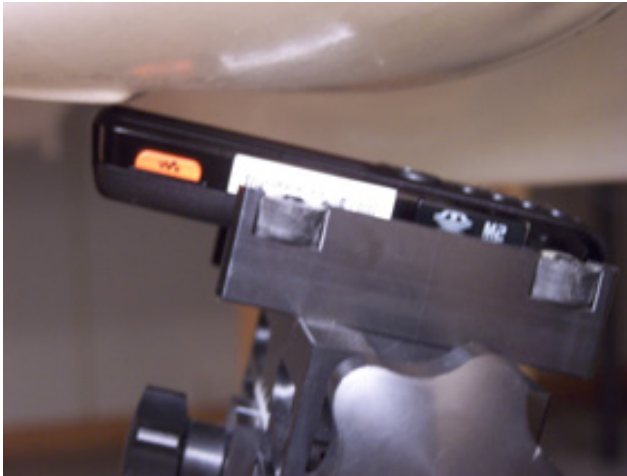
Device position against the head: Tilt (cheek+15deg) phone position
