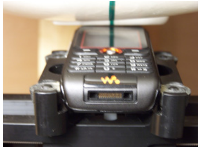
Device position against the head: Tilt (cheek+15deg) phone position
