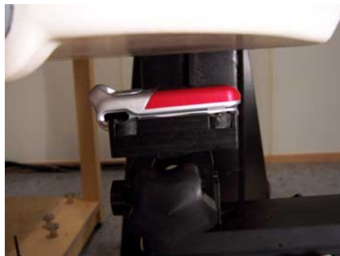
Device position against the body: phone with 15mm distance against flat section of the Phantom
