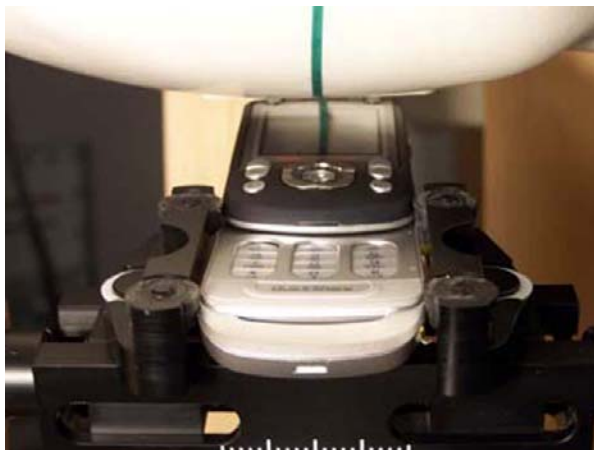
Device position against the head: Tilt (cheek+15deg) phone position (phone in open state)
