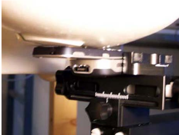
Device position against the head: Cheek (touch) phone position (phone in open state)
