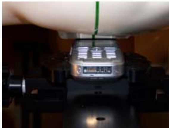
Device position against the head: Tilt phone position
