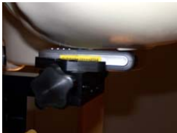
Device position against the head: Tilt phone position
