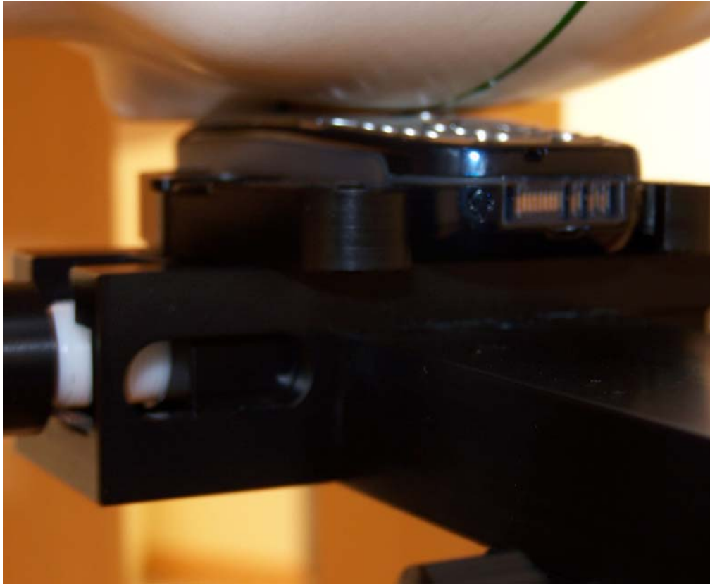
Device position against the head: Cheek phone position
