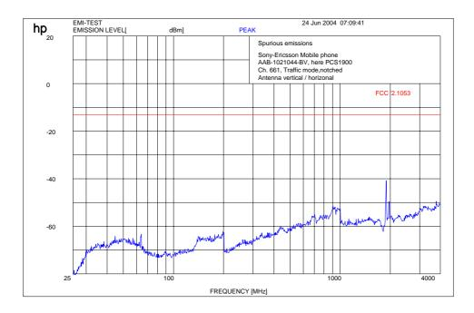
The carrier at 2 GHz is from base station simulator
