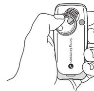
Slide the lens cover anti-clockwise to open the cover.
