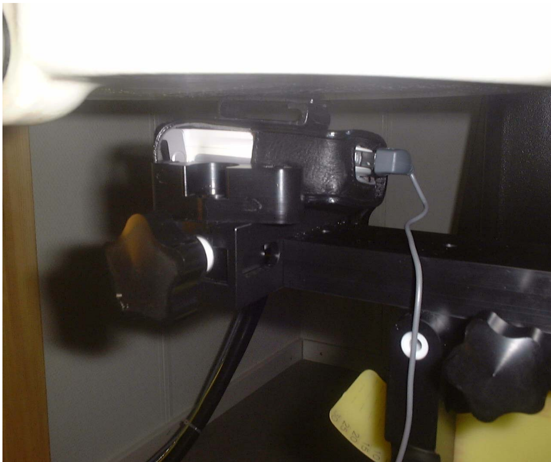
Device position against the body: Phone with belt holder under phantom and hand free connection.
