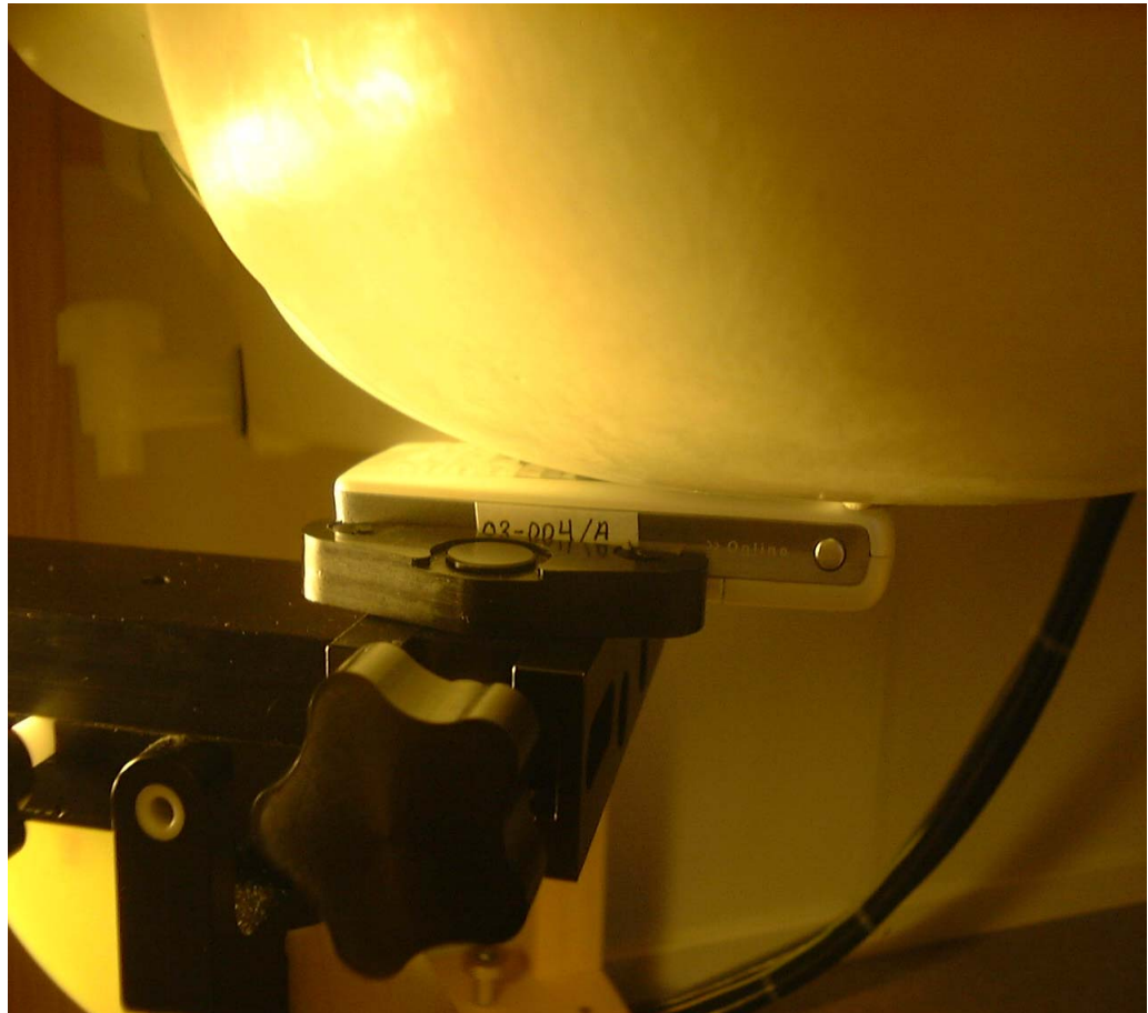
Device position against the head: Cheek (touch) phone position
