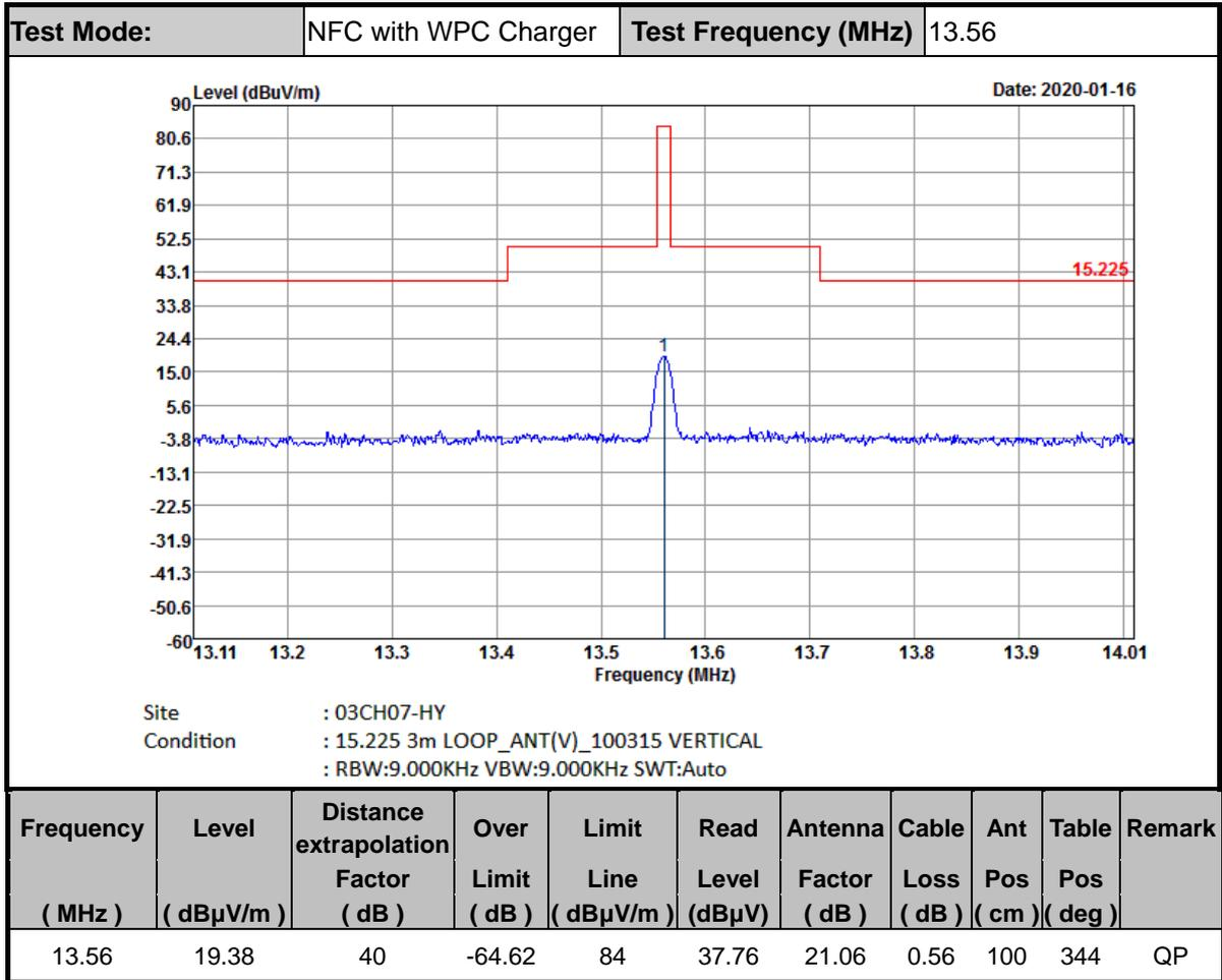
**A2. Results of Radiated Spurious Emissions (9 kHz~30MHz)**
