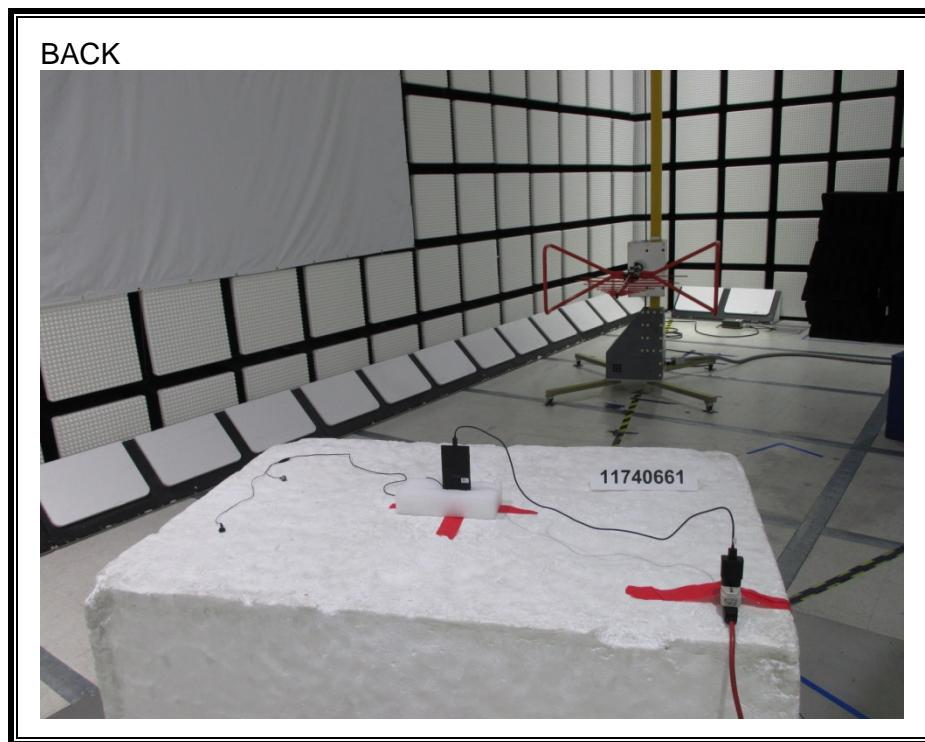
**RADIATED RF MEASUREMENT SETUP (ABOVE 1 GHz)**
