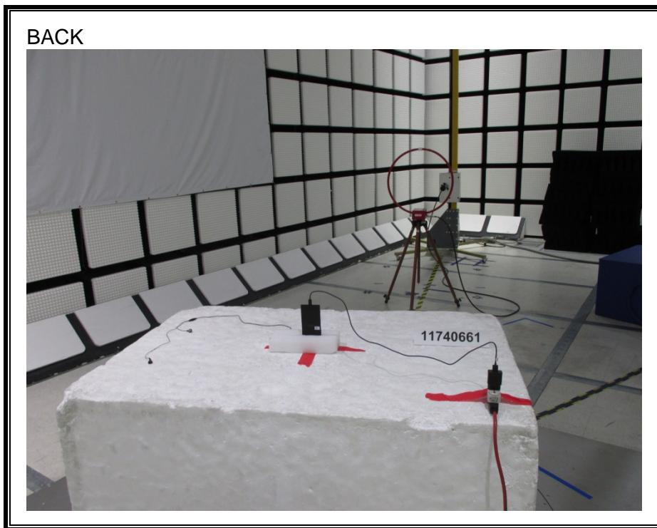
**RADIATED RF MEASUREMENT SETUP (BELOW 1 GHz)**
