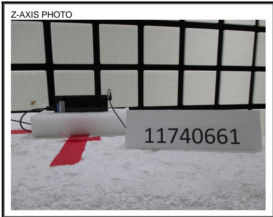
**AC LINE CONDUCTED EMISSIONS MEASUREMENT SETUP**
