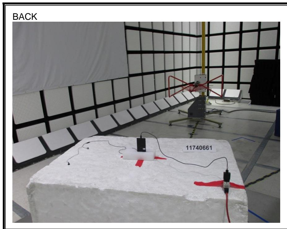
**RADIATED RF MEASUREMENT SETUP (ABOVE 1 GHz)**
