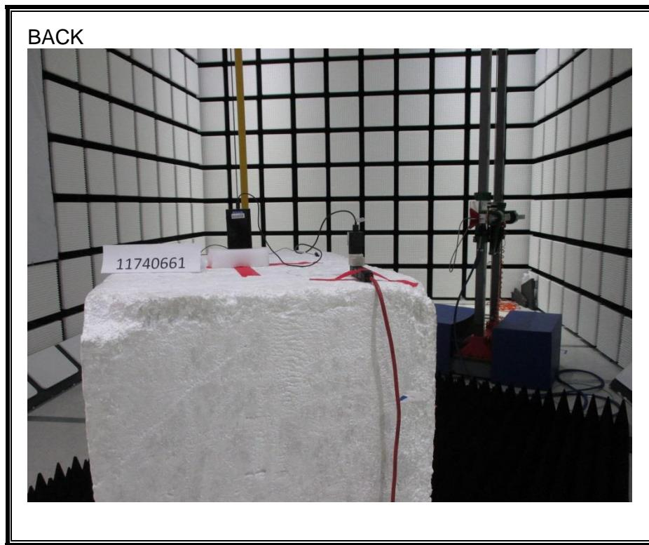
**RADIATED RF MEASUREMENT SETUP FOR PORTABLE CONFIGURATION**
