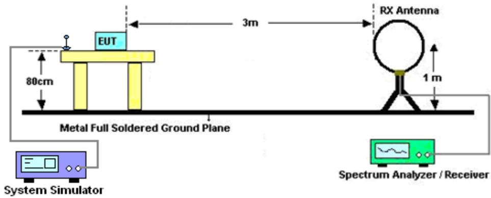
For radiated emissions from 30MHz to 1GHz
