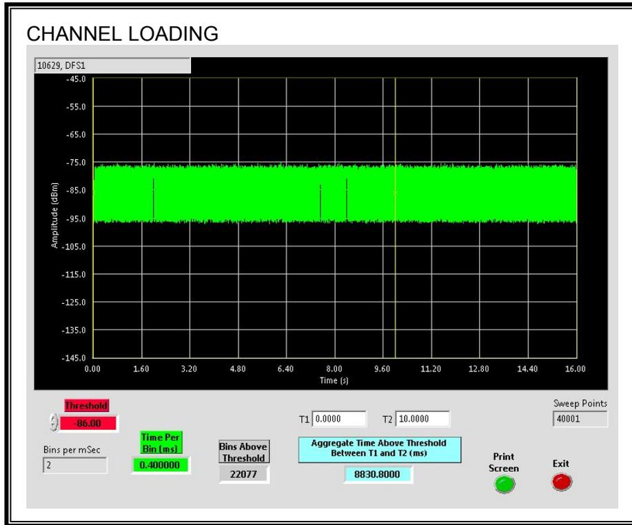
The level of traffic loading on the channel by the EUT is 88.308%.
