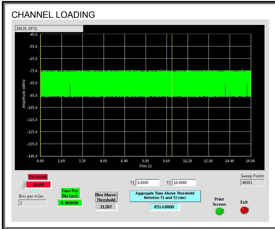
The level of traffic loading on the channel by the EUT is 85.148%.
