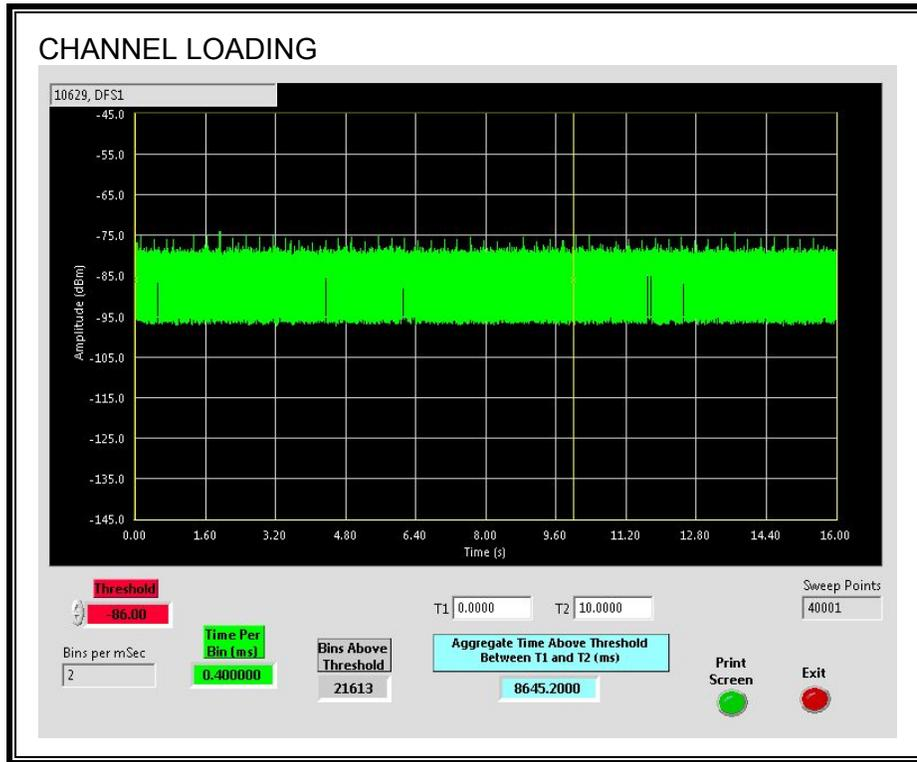
The level of traffic loading on the channel by the EUT is 86.452%.
