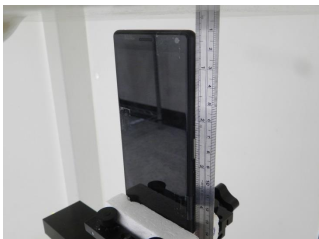
Top Side, Test Separation 10 mm
