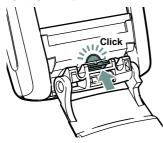
Attach the cover plate by first placing the small hooks by the screen and then press on the curved front part until it is securely fixed.
