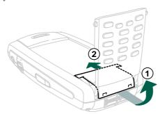
2. Unlock the catch and lift away the keypad.
