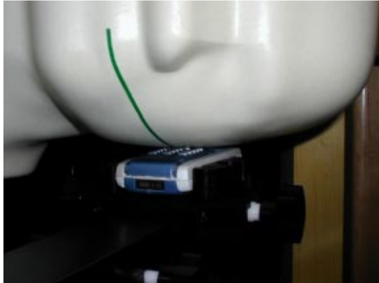
The P800 with flip on head phantom in the cheek position.
