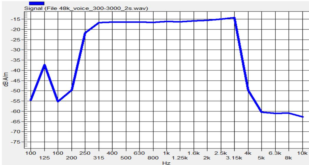
**Fig. 5.6 Audio signal spectrum of the broadband signal (48kHz\_voice\_300Hz~3 kHz)**
