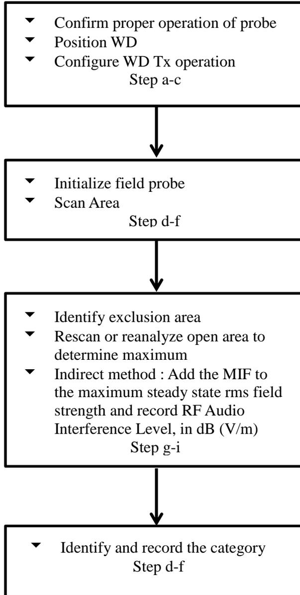
Fig 8.1 Flow Chart of HAC RF Emission
