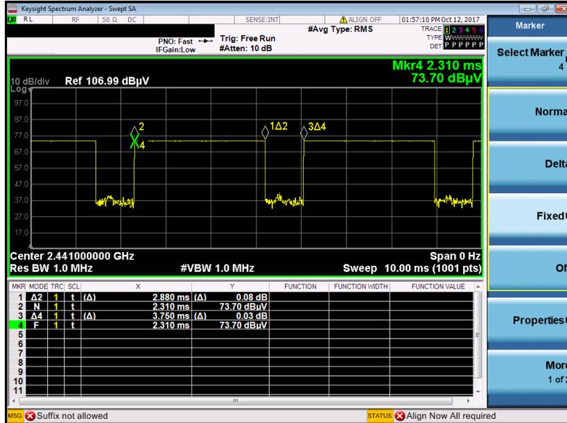
on time (Count Pulses) Plot on Channel 39
