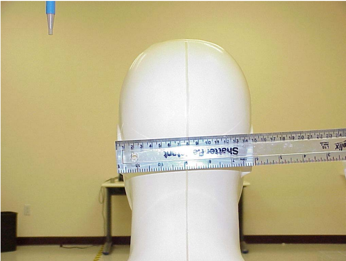
Photo 8. Photo to demonstrate 15 cm Z-axis head phantom
