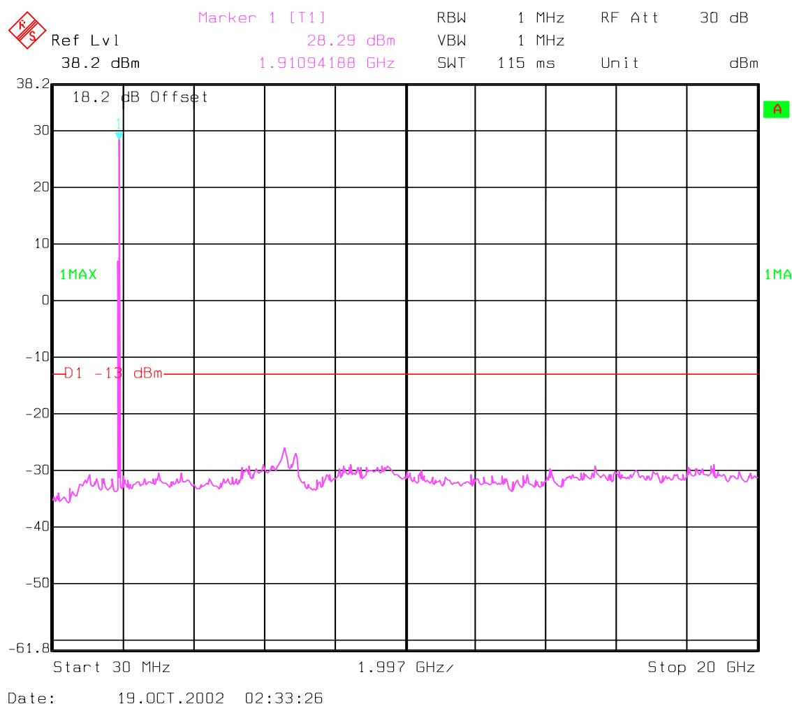
**CONDUCTED SPURIOUS EMISSIONS****Idle mode: 30MHz – 20GHz**
