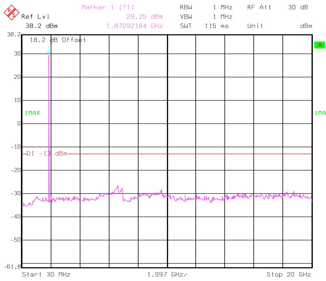
**CONDUCTED SPURIOUS EMISSIONS****Channel 810: 30MHz – 20GHz**
