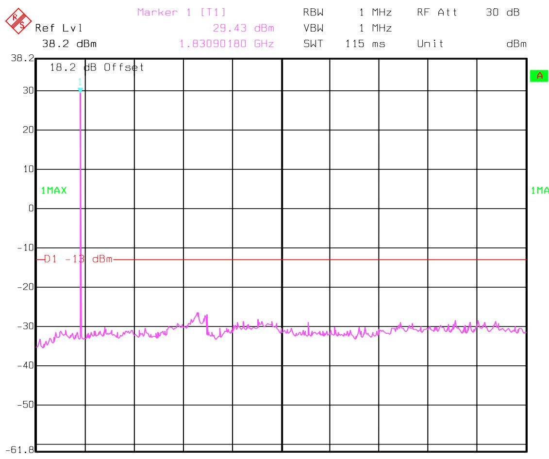
**CONDUCTED SPURIOUS EMISSIONS****Channel 661: 30MHz – 20GHz**
