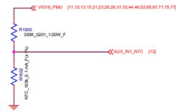
**Thermistor / To sense board level temperature**
