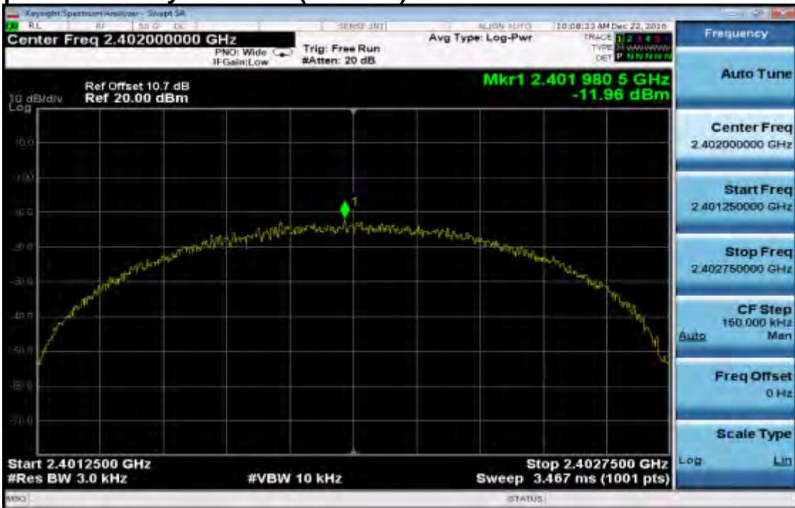
Power Spectral Density Test Plot (CH-Mid)
