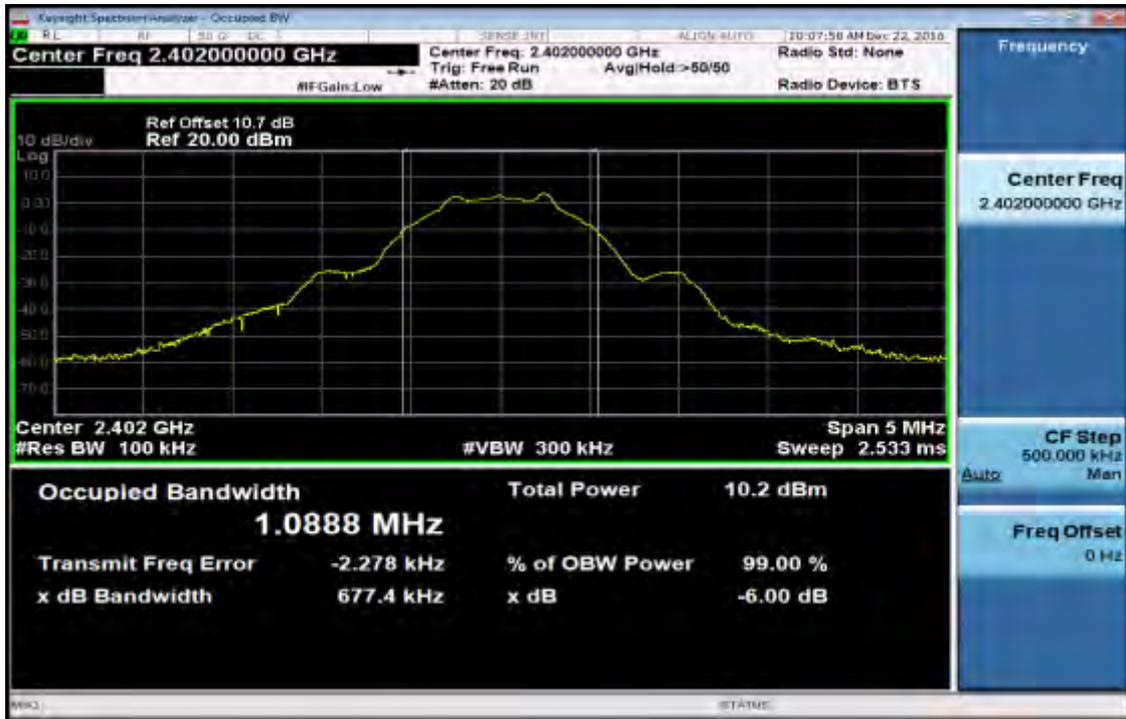
**6dB Band Width Test Data CH-Mid**
