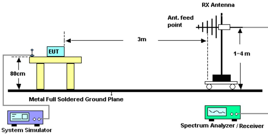
For radiated test above 1GHz
