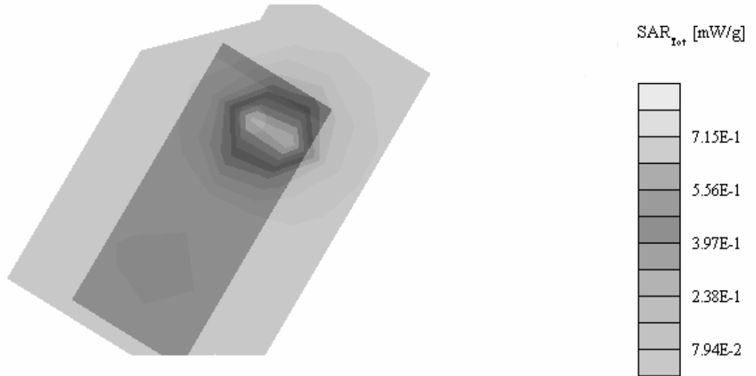
Distributions of max SAR in GSM1900 mode at 1850.2MHz. Measured against the head for tilt phone position
